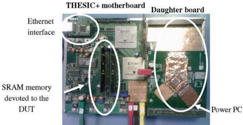
Fig. 7.16 Power PC's daughterboard plugged on THESIC + tester
