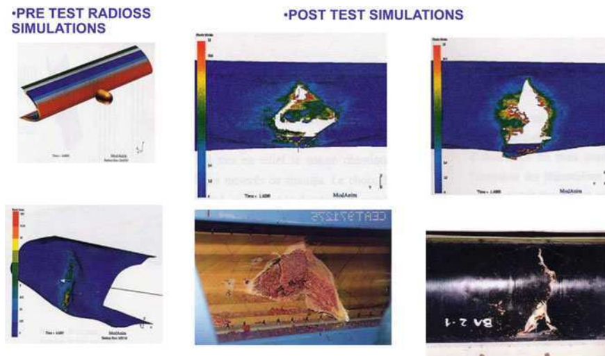
Fig. 6.6 Bird strike analysis and test comparison [17]
