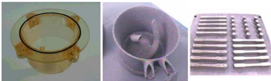
Fig. 9.9 Examples of RP adoption in industrial engineering: a component of a garment printer, a coffee machine, and some SLS specimens still on the build platform
