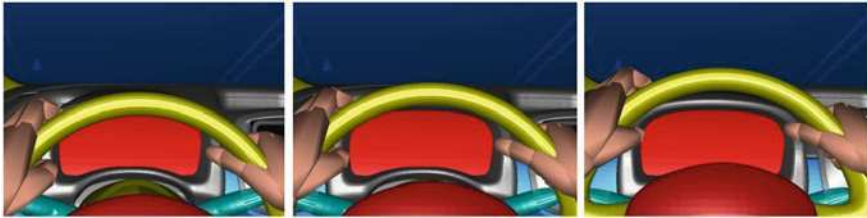
Fig. 8.4 Instruments panel visibility for a 50th percentile: seat at foremost position and steering at the three different positions
