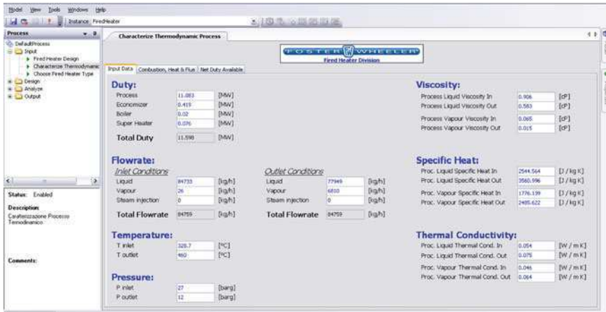
Fig. 4.13 The KB application: entering design specs for thermodynamic characterization
