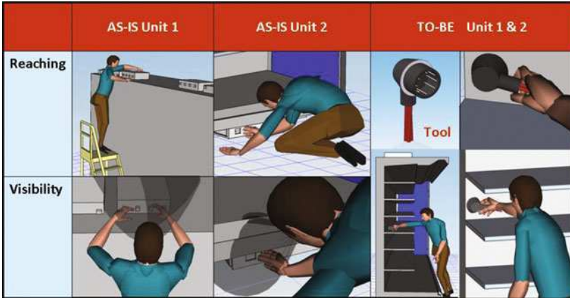
Fig. 8.12 As-Is and To-Be configuration for electric equipment
