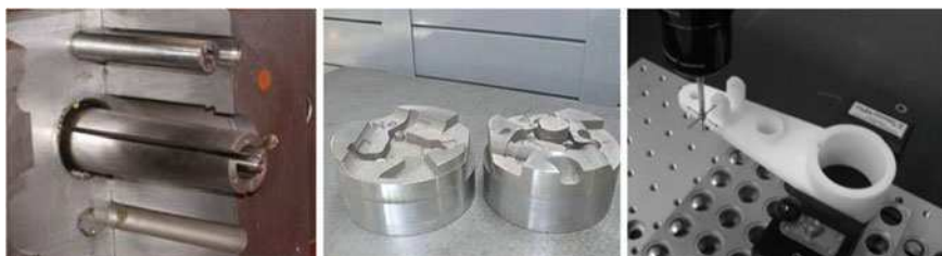
Fig. 9.10 Examples of RP adoption in industrial engineering: a mold insert for plastic injection, the mold of a camera tripod component and a mechanical component in a coordinate measuring machine
