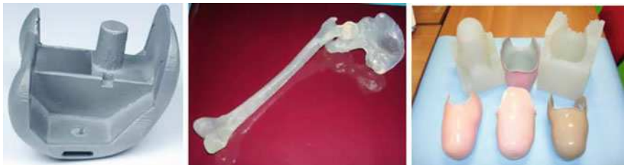
Fig. 9.8 Examples of RP adoption in medical fields: a component of knee prosthesis, a femur and part of a pelvis, and some soft sockets for lower-limb prostheses
