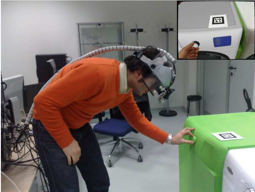
Fig. 7.8 Virtual washing machine based on MR technologies
