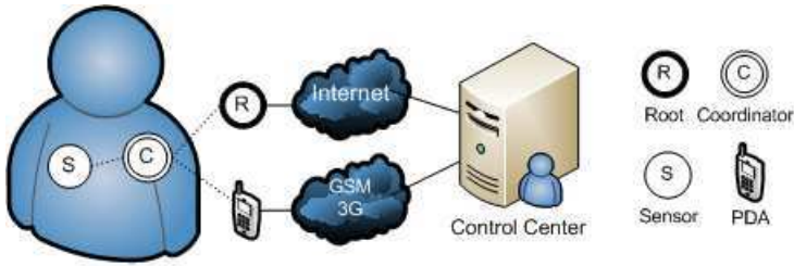
Fig. 1 The Body Monitor Architecture
