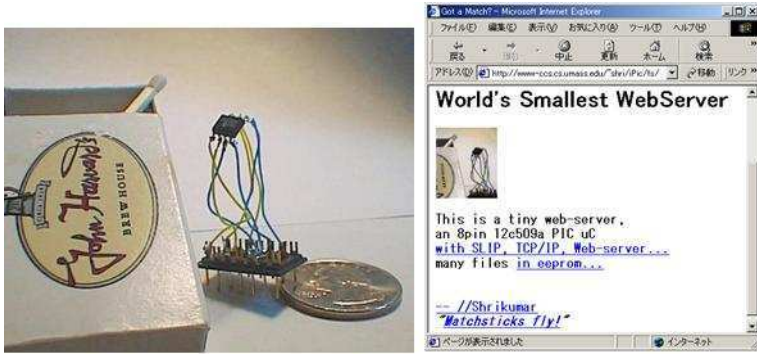
Fig. 1 iPic web-server ( http://www-ccs.cs.umass.edu/~shri/iPic.html/ ). The one-chip CPU in the left picture worked as a Web server as shown in the right picture. This site is currently closed.
