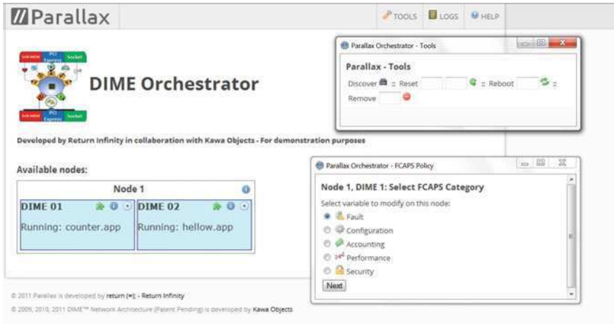
Fig. 4.6 DIME network orchestrator screenshot showing the status of two DIMEs running two different applications running on Parallax operating system in a multi-core server (A video demonstrates the input/output redirection, self-repair and auto-scaling features supported by Parallax http://youtu.be/IMXxmRSVGol )
