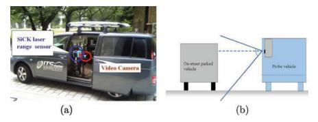
Fig.1 System configuration
