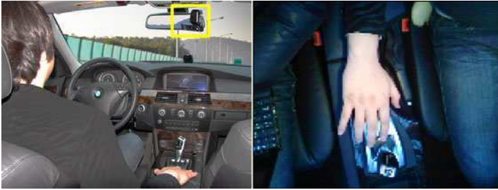
Fig. 1 (a) Camera arrangement of hand gesture control system and (b) hand image from the camera
