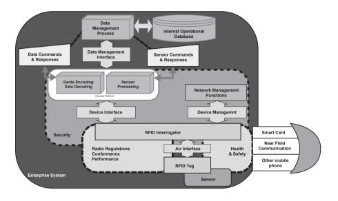
The basic RFID Device and Process Architecture is illustrated in the following graph:<sup>21</sup>
