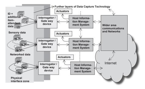
Note: Sensor-RFID structures may be distinguished that (1) allow communication simply with host readers (2) between sensor devices (dotted lines)<sup>98</sup>
