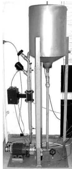
Fig. 6.14. Photo of the investigated centrifugal pump-pipe-tank plant
