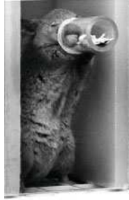
Fig. 1. Mouse reaching for food with right forepaw in unbiased U-world [24]. In U-world, food tube is centered in face of test chamber; in biased R-world or L-world, food tube is directly next to the respective right or left side from the perspective of the mouse. (Reproduced with permission from NRC Research Press. (c) 2008 NRC Canada or its licensors.)
