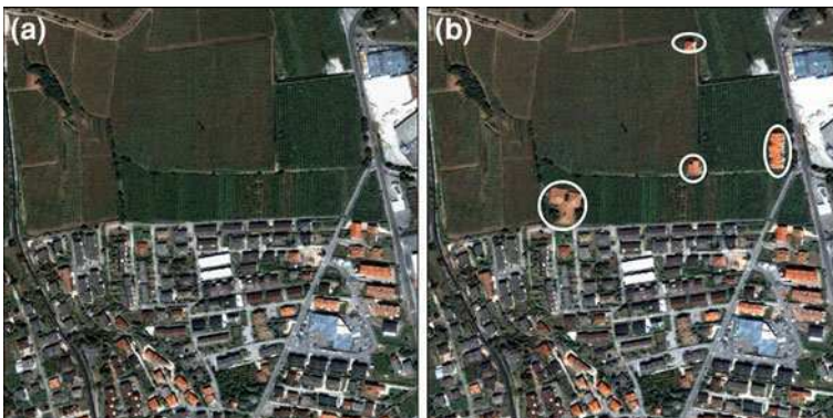
Fig. 2 Channel 4 of pan-sharpened image of the city of Trento (Italy) acquired by the Quickbird VHR multispectral sensor in July 2006 a original image without simulated changes, b original image with simulated changes (pointed out with white circles )
