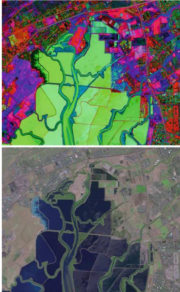
Fig. 2 Images are projections of a 224-band AVIRIS image of Moffet field [14]. Top Standard PCA visualization. Bottom Cosine-basis function visualization adapted with principal components as described in Sect. 3
