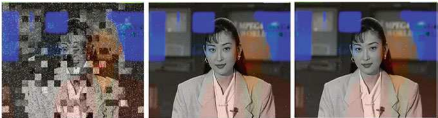
Fig. 8.21 Output video image of 32 Kbit (a) SRAM array with 6T-only cells at FS corner and V_{dd} = 600 mV, PSNR = 15.27 dB, (b) hybrid SRAM array at V_{dd} = 600 mV and FS corner, PSNR = 23.61 dB and (c) hybrid SRAM array at V_{dd} = 600 mV and SF corner, PSNR = 23.90 dB
