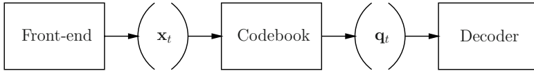
Fig. 2.11 Block diagram of the SCHMM-based speech recognizer used for the experiments of this book. A feature vector representation of the speech signal is extracted in the front-end of the speech recognizer. Each feature vector is compared with all Gaussian densities of the codebook. The result is used for speech decoding to generate a transcription of the spoken phrase. Figure is taken from [Herbig et al., 2010c].
