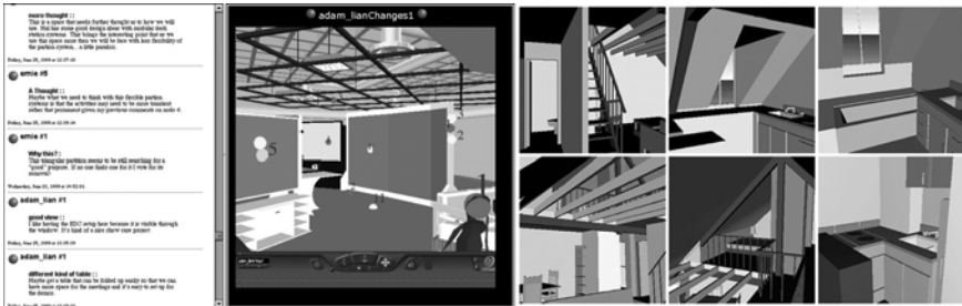
Fig. 7. Left: Redliner showing comments and annotation markers in the space. Right: Providing different design alternatives and viewpoints in apartment remodeling.
