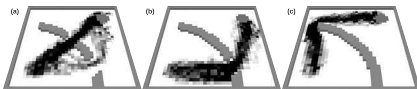
Fig. 4 Simulation of a robot swarm using the slime-mould-inspired algorithm showing the cumulative paths of loaded robots from the dirt area in lower left corner of the arena to the dump area in the upper right corner of the arena. (a) First the swarm selects the shortest path through the central door in the barrier, only a small fraction of the swarm chooses the second door which allows a slightly longer way from dirt to dump. (b) After the central door was closed, the swarm automatically selects the lower door which offers now the shortest path. (c) After this door was closed too, the swarm chooses the only remaining longest path. Reprinted from [26].
