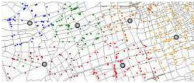
Fig. 1. Distribution of hot terminals (6 black points) in rebuilt map based on real pick-up (colored points belong to its closest hot terminals) data
