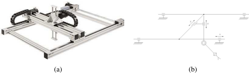
Fig. 2. Institutions and joint composition of Cartesian type manipulator
