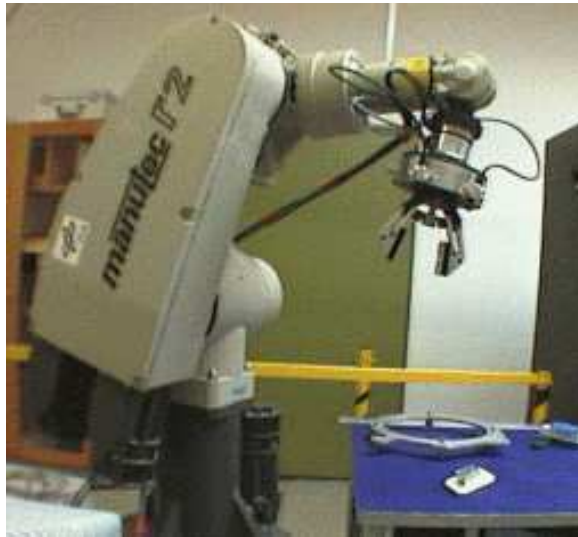
Figure 3: Real time visual servoing for robot grasping
