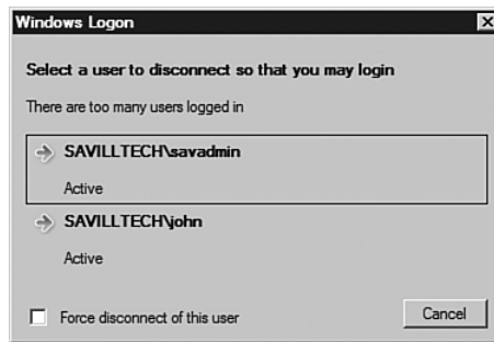
FIGURE 9-8 Even if a server is full, you can now connect by disconnecting an existing session.
