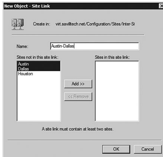
FIGURE 12-3 You can configure some basic properties via the New Object - Site Link dialog.
