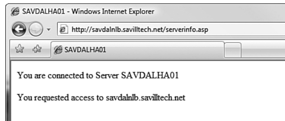
FIGURE 18-10 A test page showing which server handled a request and the URL entered by the user.
