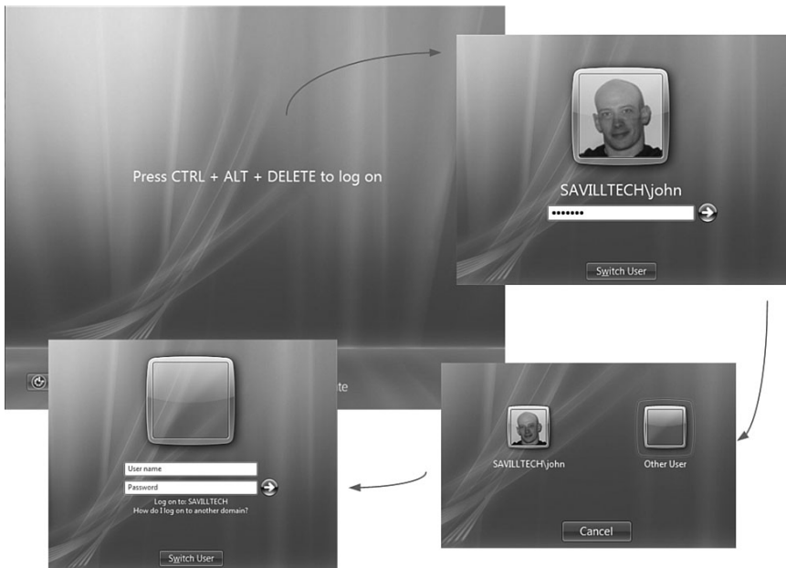
FIGURE 2-4 In the Windows Vista and Windows Server 2008 logon process for a domain-joined machine, you have a Switch User option.
