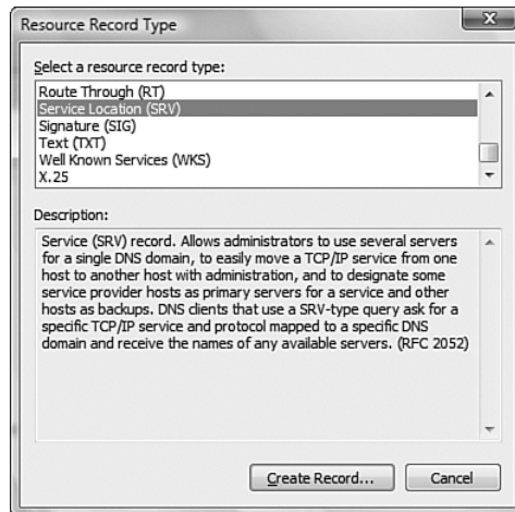
FIGURE 7-37 A lot of DNS record types exist; here, you see the service record type along with its description.
