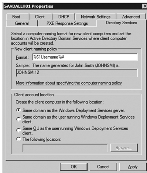
FIGURE 16-19 The naming scheme used for the computer and the computer object's creation location.
