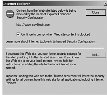
FIGURE 4-40 The IE ESC message for a site trying to run content that is blocked by IE ESC.
