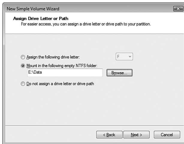
FIGURE 5-5 In this example, the new volume is available as a subfolder of the existing E: drive.
