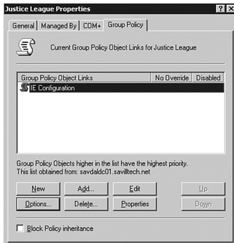
FIGURE 21-14 Hopefully you never have to use this. This shows the GPOs that are linked to a container.
