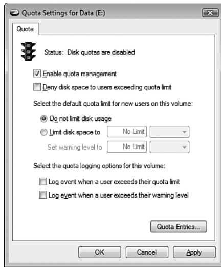
FIGURE 5-16 The quota allows disk space usage to be limited to a certain predefined amount.
