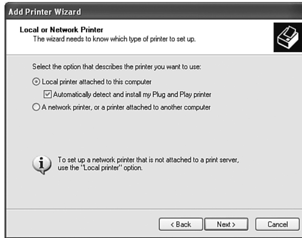
FIGURE 5-69 Selection of the XP printer. For a printer on a print server, select the second option.
