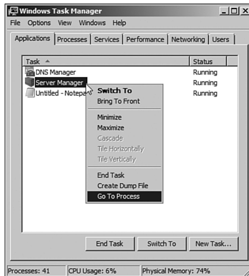
FIGURE 2-25 The Applications tab shows all running applications. Select an application and stop it by clicking End Task, give it the focus by clicking Switch To, or right-click for additional options.
