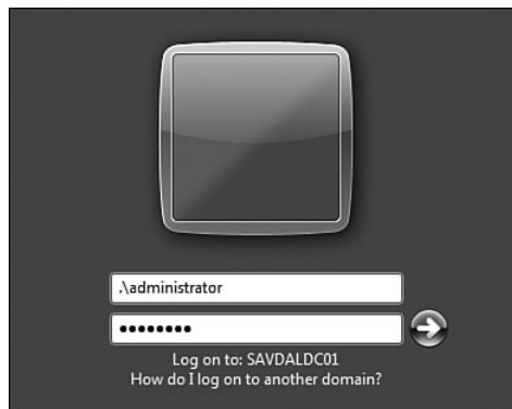
FIGURE 12-37 The .\ tells the system to use the local account database for logon.
