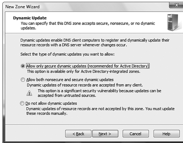
FIGURE 7-43 Disable dynamic update so all records must be manually created, or enable in a secure or nonsecure form.
