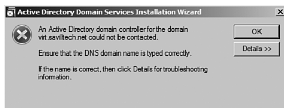
FIGURE 12-10 Connectivity to the forest root is needed to demote a domain controller.
