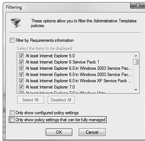
FIGURE 21-84 Make sure Only Show Policy Settings That Can Be Fully Managed is unchecked.
