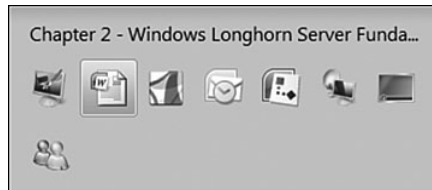
FIGURE 2-15 The standard Alt+Tab list displays the shortcut icon for each running application, allowing for keyboard-based switching between applications.
