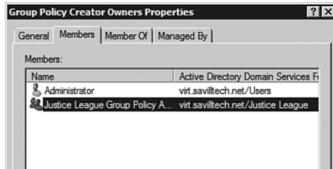
FIGURE 21-70 This group is an easy and supported way to give non-administrators the capability to create GPOs.
