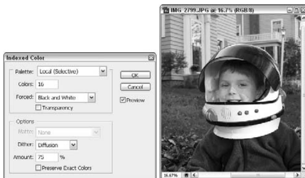
Figure 3-4: Index color uses a limited number of colors to create an image.
