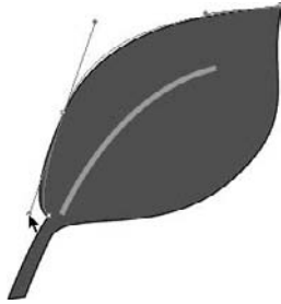
Figure 5-1: The depth and direction of the Bézier curves are controlled by direction lines.
