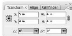
Figure 4-6: Use the Transform panel to precisely set the size of a shape.
