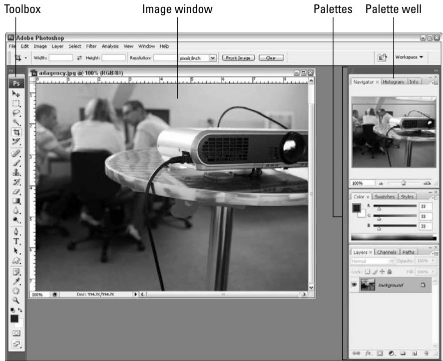
Figure 2-1: Photoshop CS3 workspace includes the toolbox, palettes, and palette well.
