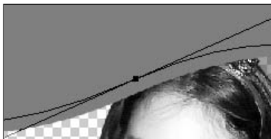
Figure 5-6: Edit individual anchor points with the Direct Selection tool.
