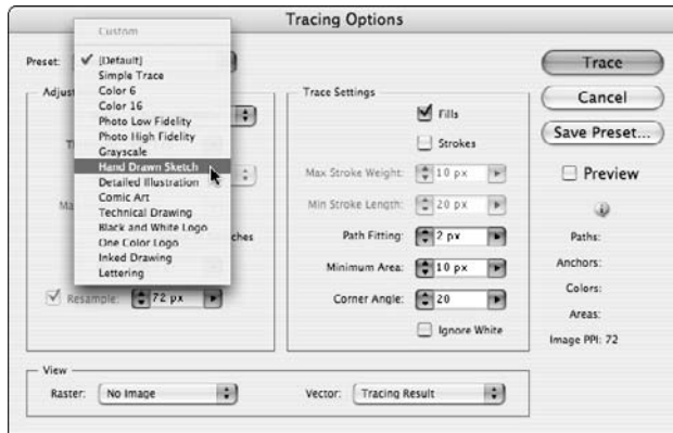
Figure 9-17: Turn bitmap artwork into vector using the Live Trace feature.
