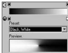
Figure 4-11: The gradient pop-up window has controls for color and opacity, a list of gradient presets, and a Preview pane.
