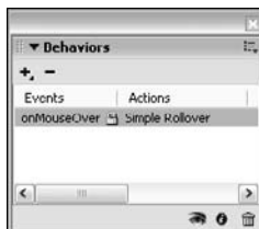
Figure 7-9: The Behaviors panel shows the action(s) assigned to a slice.
