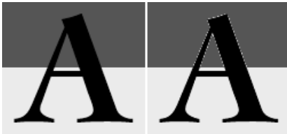
Figure 7-1. Using PNG or the <canvas> tag, edges are clean no matter what background the image is superimposed on, whereas quality is poor with GIF
