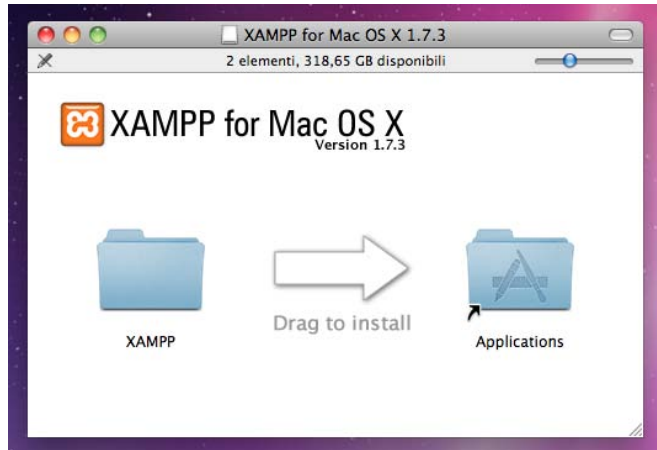
Figure 9-4. Just drag the XAMPP DMG file to the Applications folder on your Mac to install the server.
