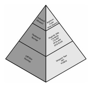
As one goes down the hierarchy: (a) decreasing cost per bit; (b) increasing capacity; (c) increasing access time; (d) decreasing frequency of access of the memory by the processor.
