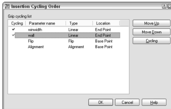
Figure 2-8: Defining insertion cycling for a block can make inserting it easier.
