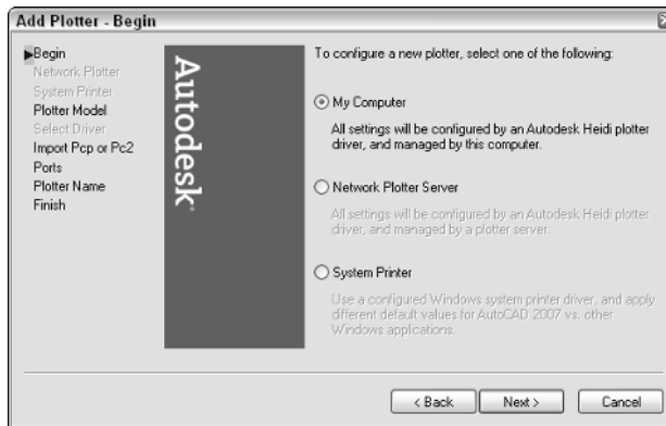
Figure 3-2: The Add Plotter Wizard is used to configure a non-system printer.
