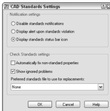
Figure 2-3: Fine-tuning the behavior of the CAD standards tools.
