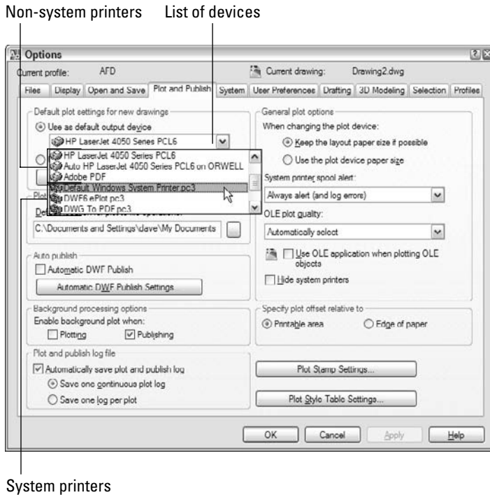
Figure 13-1: System and non-system printer con- figurations.
