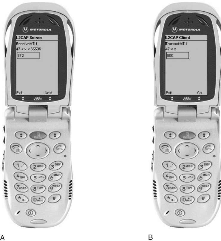
Figure 8.4 User interface for MTU experiments. (A) A receiveMTU of 672 bytes is entered for the server. (B) A transmitMTU of 500 bytes is entered for the client (emulation only).
