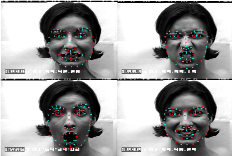
Fig. 5. Examples of old (red circle) and new (cyan cross) FFPs in CK+ database (Images of 1 subject with 4 expressions)
