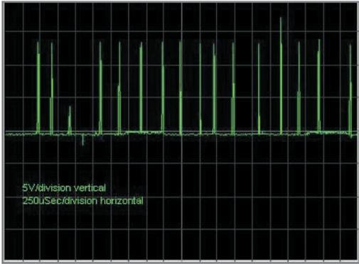
**Photo 3**—This is the close-up view of the MOSFET's gate drive at 5 V with a 0.5-A load. The load is light, so the MOSFET's gate drive is not regular. The gate drive is just enough to keep the voltage at 5 V and the current at 500 mA.
