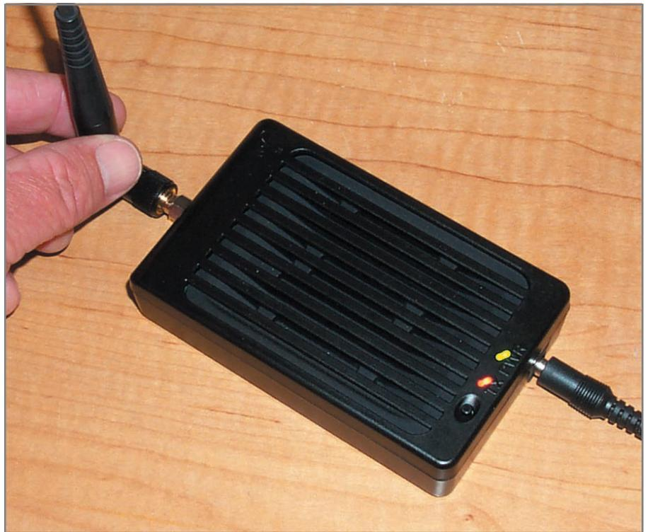
**Photo 5**—There’s more to antenna gain than just the type of antenna. A faulty implementation (e.g., impedance mismatch) can cause a loss of efficiency or even damage the transmitter. Here the red LED on the transmitter indicates it has shut down, having detected something is amiss.
