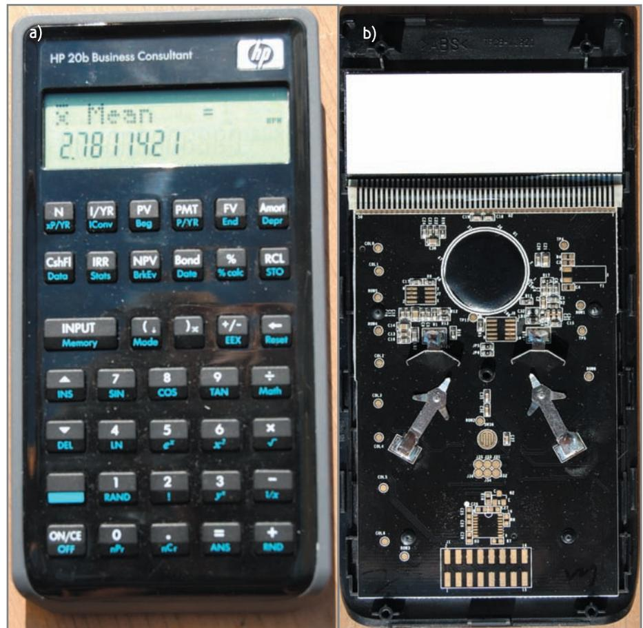
**Photo 1a**—This is the HP20b calculator. **b**—The HP20b, inside out! The Atmel microprocessor is hiding under the Bakelite “blob” and the JTAG connector at the bottom.
