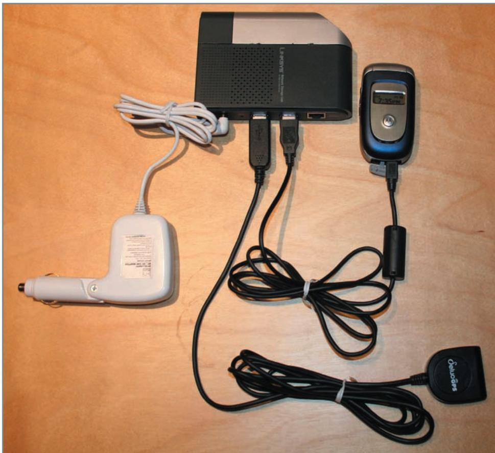
**Photo 1**—The assembled vehicle locator includes a Linksys WLU2 USB Network storage link, a Motorola GSM phone, and a Deluo USB-GPS device.
