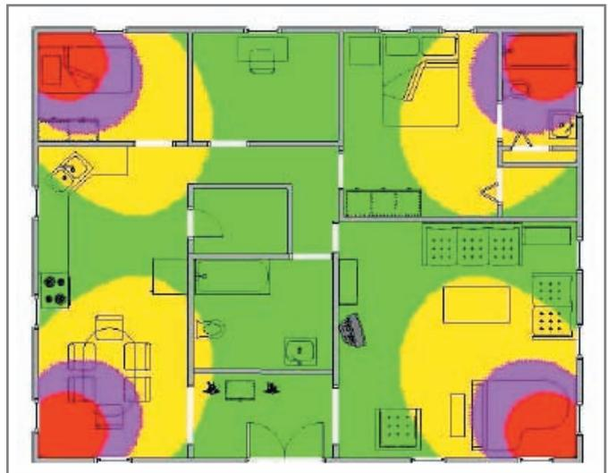
**Figure 3**—Like a cell phone network, multiple transmitters can help ensure full coverage, a must in situations where receivers may move around or be blocked by transient obstacles, such as people wandering around.
