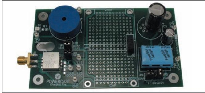
**Photo 2**—PowerCast offers an evaluation board that uses a P2100 harvester to “charge and fire” the 0.22F supercap located on the lower right side of the board.
