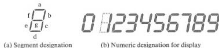
□ FIGURE 3-12 Seven-Segment Display
