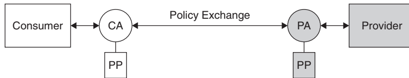
FIGURE 29.8 Exchange of privacy policies (PP) between consumer agent (CA) and provider agent (PA).
