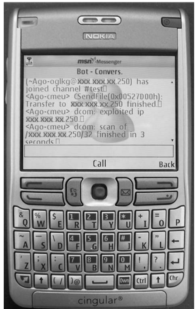
FIGURE 8.8 Using a Nokia smartphone to control an Agobot-based botnet. (Photo courtesy of Ruishan Zhang.)
