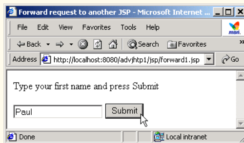
Fig. 10.11 JSP forward1.jsp receives a firstName parameter, adds a date to the request parameters and forwards the request to forward2.jsp for further processing (part 2 of 2).
