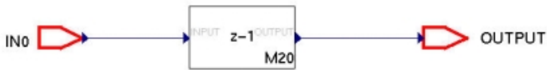
Fig. 7.6. COSSAP BDE of a 20-bit delay sub-block.
