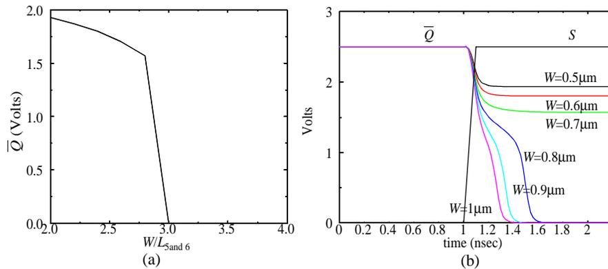
**Figure 7.9** Sizing issues for SR flip-flop. (a) DC output voltage vs. individual pull-down device size of  $M_5$  and  $M_6$  with  $W/L_2 = 1.5\mu\text{m}/.25\mu\text{m}$ . (b) Transient response shows that  $M_5$  and  $M_6$  must each have a  $W/L$  larger than 3 to switch the SR flip-flop.
