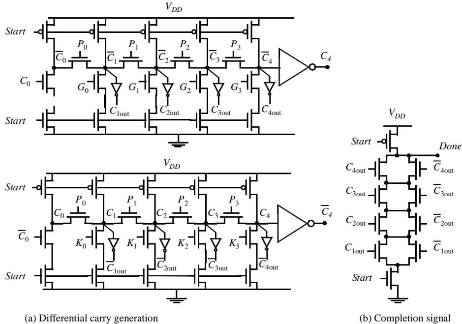
**Figure 10.34** Manchester-carry scheme with differential signal representation.
