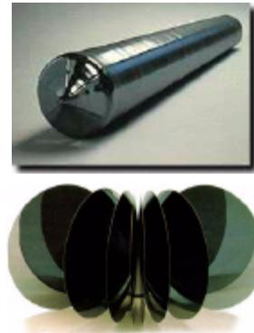
Figure 2.3 Single-crystal ingot and sliced wafers (from [Fullman99]).
