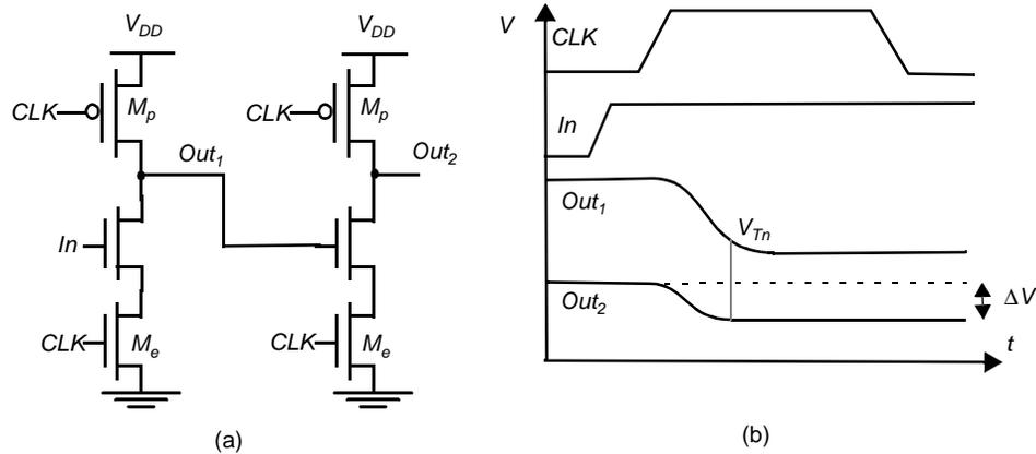
Figure 6.64 Cascade of dynamic  $n$ -type blocks.
