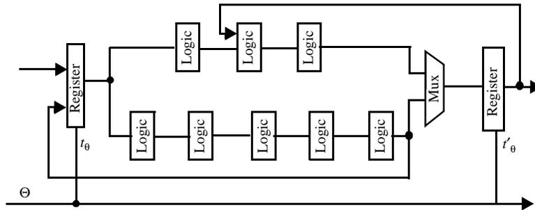
**Figure 0.1** Sequential circuit.
