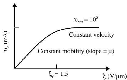
Figure 3.17 Velocity-saturation effect.
