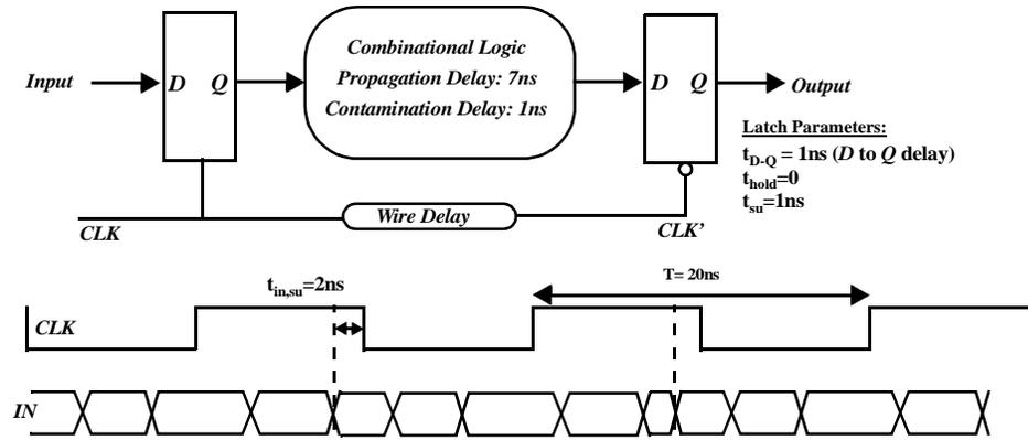
Figure 0.8 Latch based pipeline
