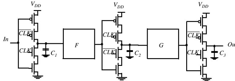
Figure 7.42 Pipelined datapath using  $C^2$ MOS latches.
