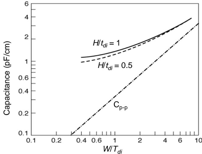
**Figure 4.5** Capacitance of interconnect wire as a function of  $(W/t_{di})$ , including fringing-field effects (from [Schaper83]). Two values of  $H/t_{di}$  are considered. Silicon-dioxide with  $\epsilon_r = 3.9$  is used as dielectric.
