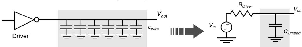
**Figure 4.11** Distributed versus lumped capacitance model of wire.  $C_{lumped} = L \times C_{wire}$ , with  $L$  the length of the wire and  $C_{wire}$  the capacitance per unit length. The driver is modeled as a voltage source and a source resistance  $R_{driver}$ .
