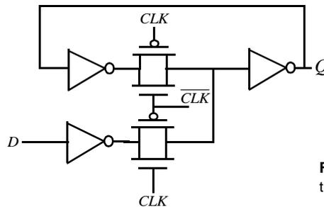
**Figure 7.12** Positive latch built using transmission gates.
