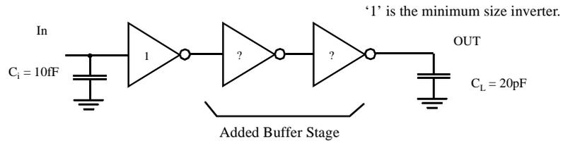
**Figure 5.12** Buffer insertion for driving large loads.
