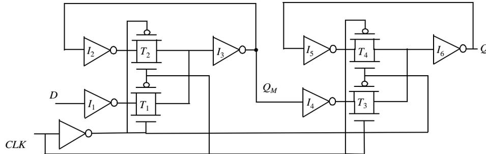
Figure 7.15 Master-slave positive edge-triggered register using multiplexers.
