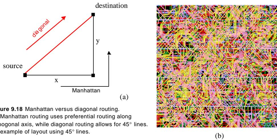
**Figure 9.18** Manhattan versus diagonal routing. (a) Manhattan routing uses preferential routing along orthogonal axis, while diagonal routing allows for 45° lines. (b) example of layout using 45° lines.
