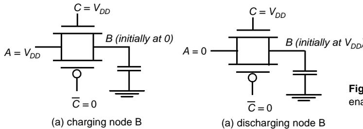
Figure 6.45 Transmission gates enable rail-to-rail switching
