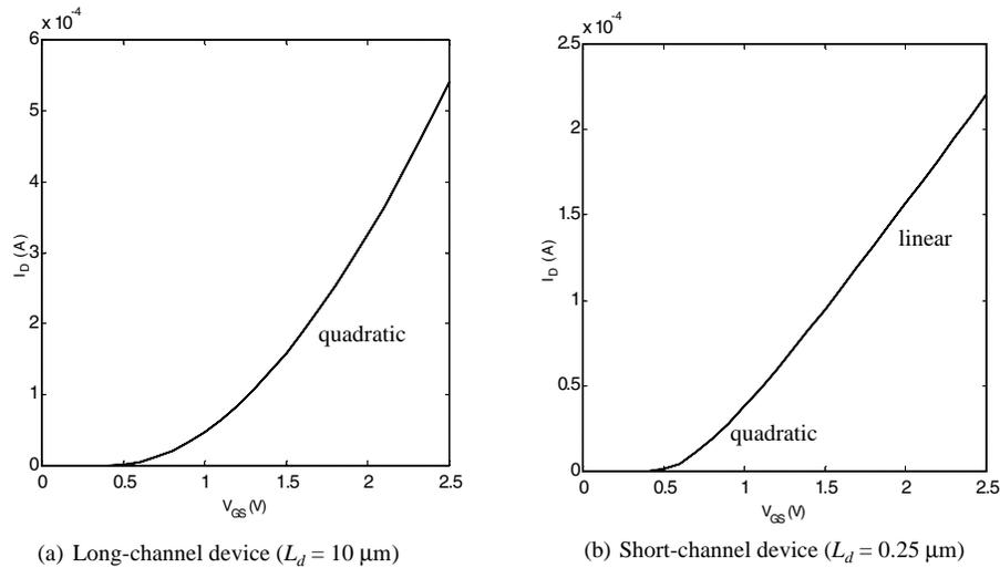
**Figure 3.20** NMOS transistor  $I_D$ - $V_{GS}$  characteristic for long and short-channel devices ( $0.25 \mu\text{m}$  CMOS technology).  $W/L = 1.5$  for both transistors and  $V_{DS} = 2.5 \text{ V}$ .
