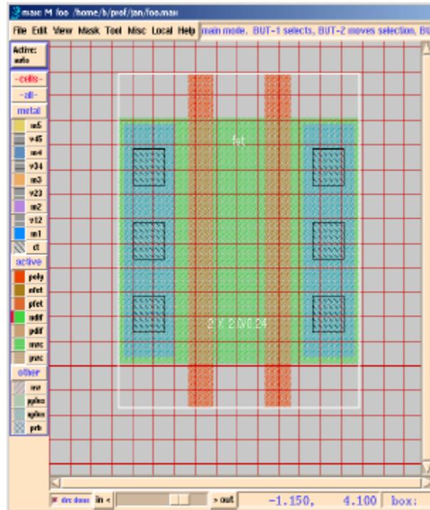
**Figure A.1** View of a **max** display window. It plots the layout of two stacked NMOS transistor. The menu on the left side allows for the selection of the layer a particular polygon will be placed on.
