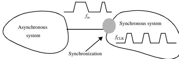
**Figure 10.50** Asynchronous-synchronous interface
