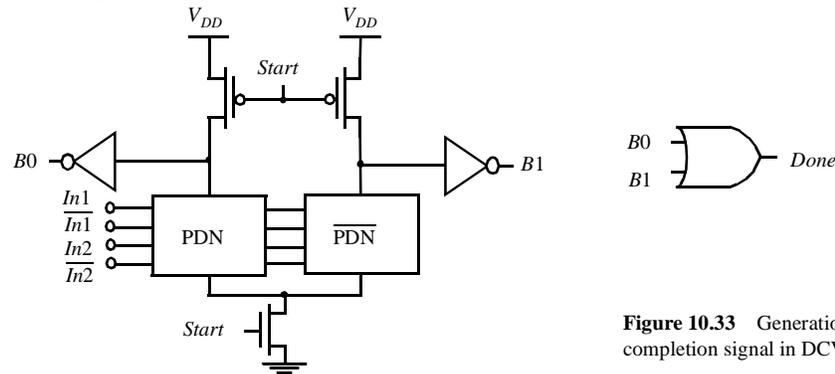
**Figure 10.33** Generation of a completion signal in DCVSL.
