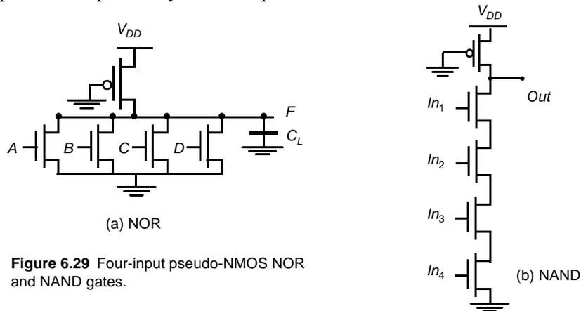
**Figure 6.29** Four-input pseudo-NMOS NOR and NAND gates.
