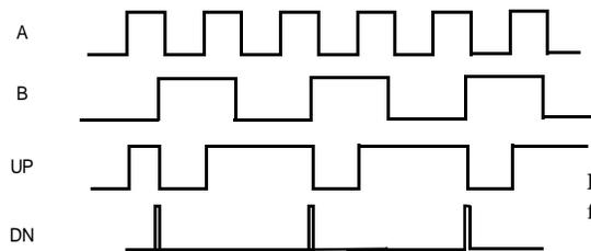
Figure 10.61 Timing of the PFD measuring frequency error.
