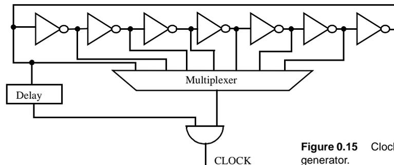
**Figure 0.15** Clock duty-cycle generator.
