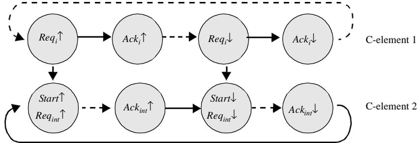
**Figure 10.45** State transition diagram for pipeline stage 1. The nodes represent the signaling events, while the arrows express dependencies. Arrows in dashed lines express actions in either the preceding or following stage.
