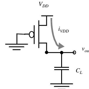
**Figure 5.25** Equivalent circuit during the low-to-high transition.
