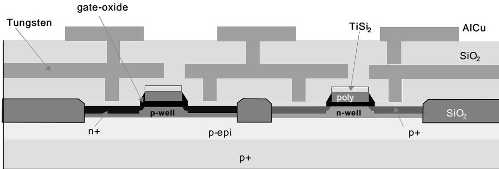
Figure 3.11 Cross-section of contemporary dual-well CMOS process.
