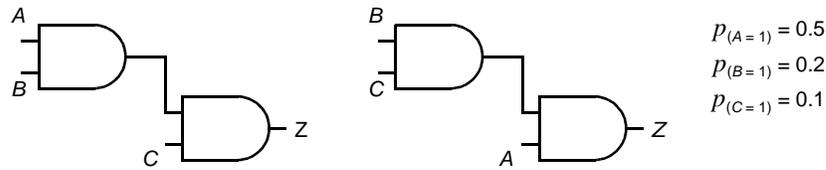
**Figure 6.24** Reordering of inputs affects the circuit activity.
