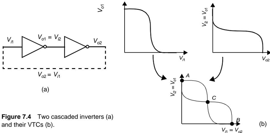
Figure 7.4 Two cascaded inverters (a) and their VTCs (b).
