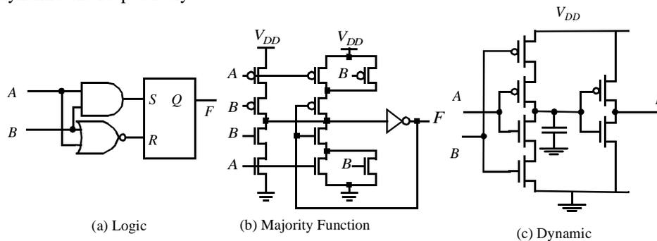
Figure 10.39 Implementations of a Muller C-element.
