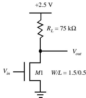
**Figure 5.3** Resistive-load inverter
