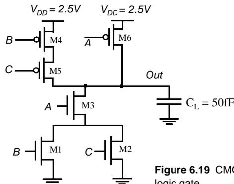
Figure 6.19 CMOS logic gate.
