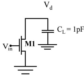
**Figure 0.10** The circuit for testing the time to discharge the load capacitance through a device operating in subthreshold region.
