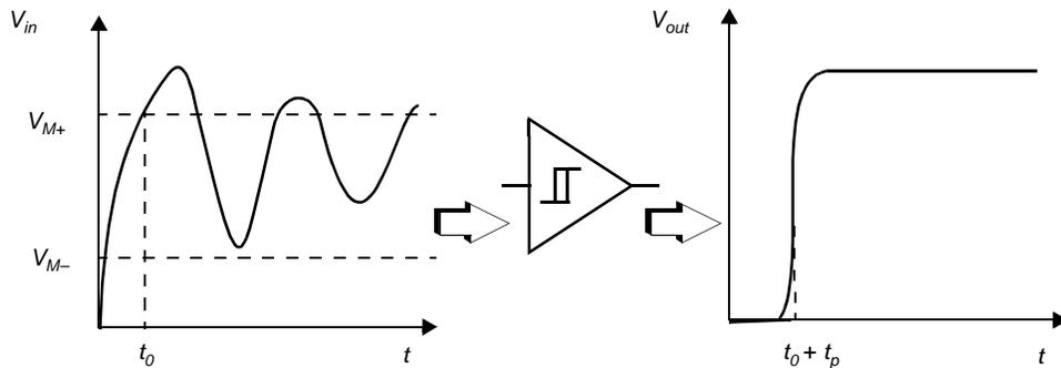
Figure 7.47 Noise suppression using a Schmitt trigger.
