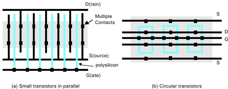
**Figure 9.8** Approaches to implementing very wide transistors.
