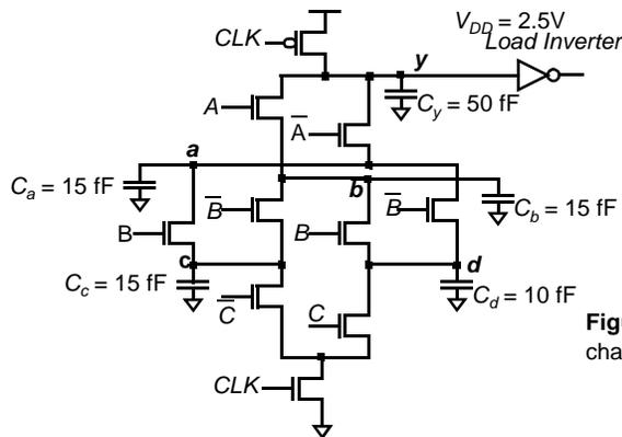
**Figure 6.60** Example illustrating the charge sharing effect in dynamic logic.
