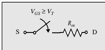
**Figure 3.25** NMOS transistor modeled as a switch.
