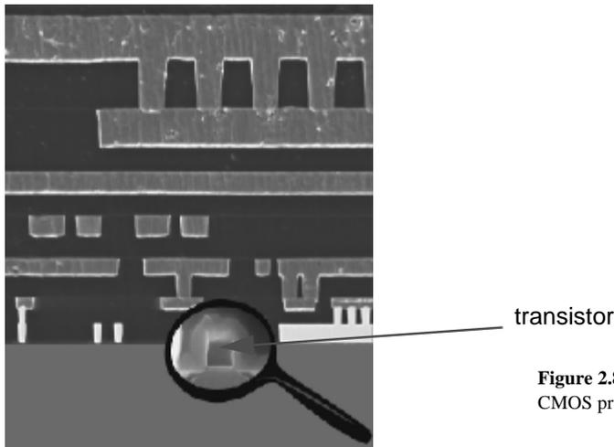
**Figure 2.8** Cross-section of state-of-the-art CMOS process.
