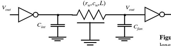
**Figure 5.24** Inverter driving single fanout through wire of length  $L$ .
