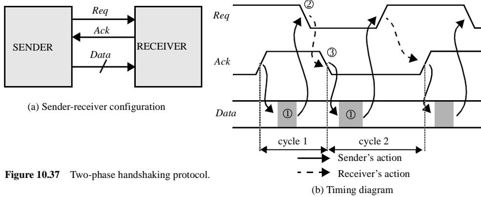
Figure 10.37 Two-phase handshaking protocol.
