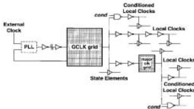
Figure 10.24 Clock hierarchy for the Alpha 21264 Processor.
