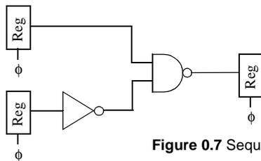
Figure 0.7 Sequential Circuit
