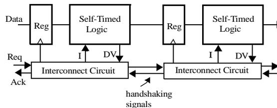
Figure 10.4 Asynchronous design methodology for simple pipeline interconnect.
