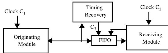
Figure 10.3 Plesiochronous communications using FIFO.
