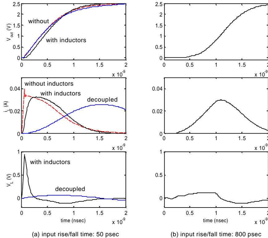
**Figure 9.22** Simulated signal waveforms for output driver connected to bonding pads for input rise/fall times of 50 psec (a) and 800 psec (b), respectively. The waveforms in (a) show the results when (1) no inductors are present in the power distribution network (ideal case); (b) in the presence of inductors; and (c) with added decoupling capacitance of 200 pF.
