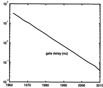
**Figure 5.39** Scaling of the gate delay (from [Dally98]).
