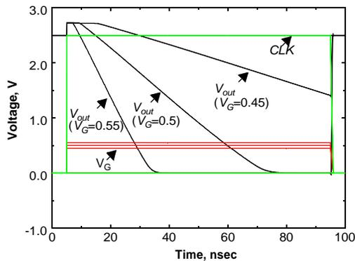
**Figure 6.54** Effect of an input glitch on the output. The switching threshold depends on the time for evaluation. A larger glitch is acceptable if the evaluation phase is smaller. In this example, the input glitches high during evaluation and stays high during the whole period.
