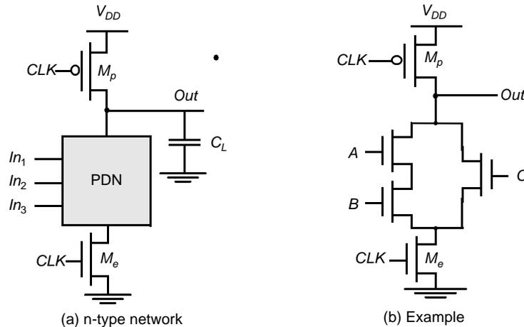
Figure 6.52 Basic concepts of a dynamic gate.
