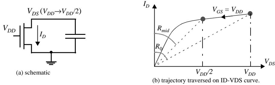
**Figure 3.26** Discharging a capacitor through an NMOS transistor: Schematic (a) and  $I$ - $V$  trajectory (b). The instantaneous resistance of the transistor equals  $(V_{DS}/I_D)$  and is visualized by the angle with respect to the  $y$ -axis.
