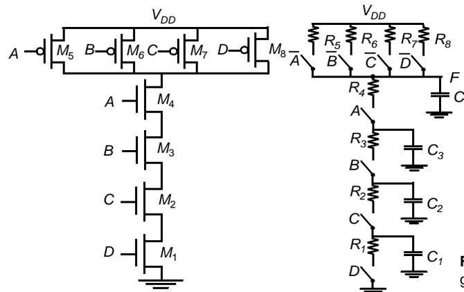
**Figure 6.11** Four input NAND gate and its RC model.
