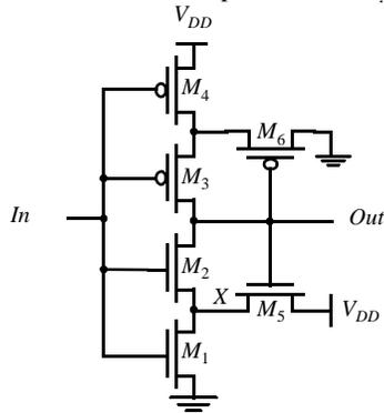
**Figure 7.50** Alternate CMOS Schmitt trigger.
