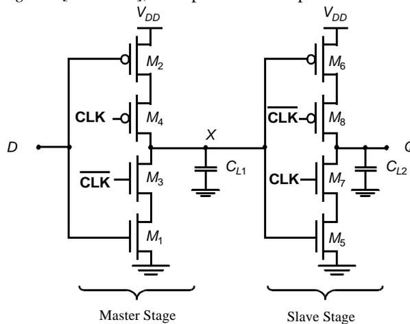
Figure 7.26 C<sup>2</sup>MOS master-slave positive edge-triggered register.
