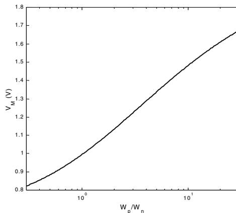
**Figure 5.7** Simulated inverter switching threshold versus PMOS/NMOS ratio (0.25  $\mu\text{m}$  CMOS,  $V_{DD} = 2.5$  V)
