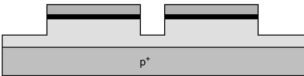
(c) After plasma etch of insulating trenches using the inverse of the active area mask
