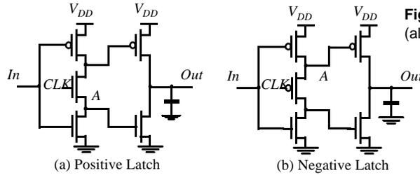
**Figure 7.32** Simplified TSPC latch (also called split-output).
