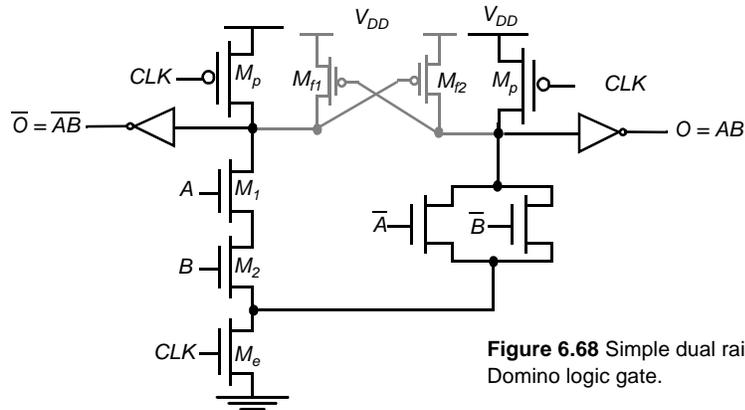
**Figure 6.68** Simple dual rail (differential) Domino logic gate.
