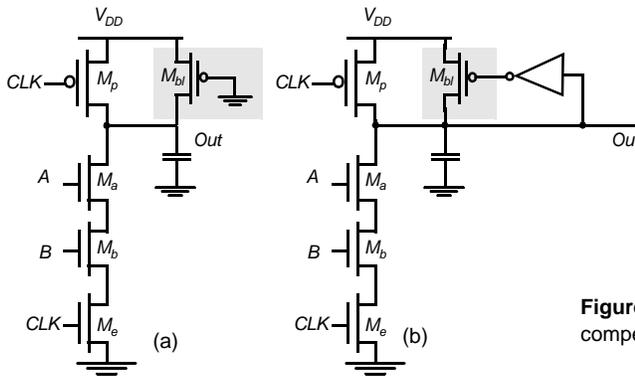
**Figure 6.58** Static bleeders compensates for the charge-leakage.
