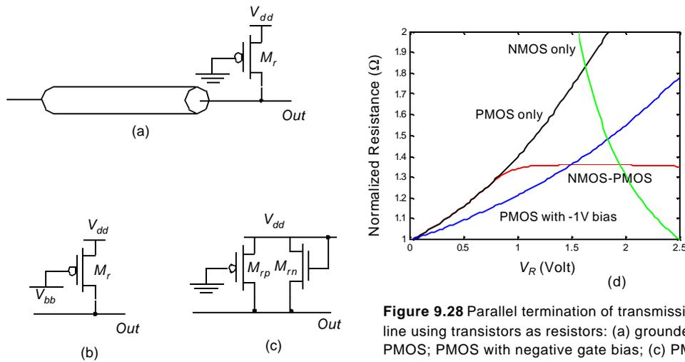
**Figure 9.28** Parallel termination of transmission line using transistors as resistors: (a) grounded PMOS; PMOS with negative gate bias; (c) PMOS-NMOS combination; (d) Simulation.
