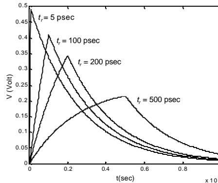
(b) Voltage response for different rise times of  $V_x$  (0 to 2.5 V) ( $R_x = 10 \text{ k}\Omega$ ,  $C_y = 20 \text{ fF}$ ,  $C_{xy} = 5 \text{ fF}$ )**Figure 9.3** Capacitive coupling to a driven line.
