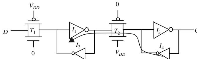
Figure 7.19 Reverse conduction possible in the transmission gate.
