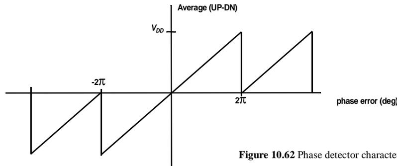
Figure 10.62 Phase detector characteristic.
