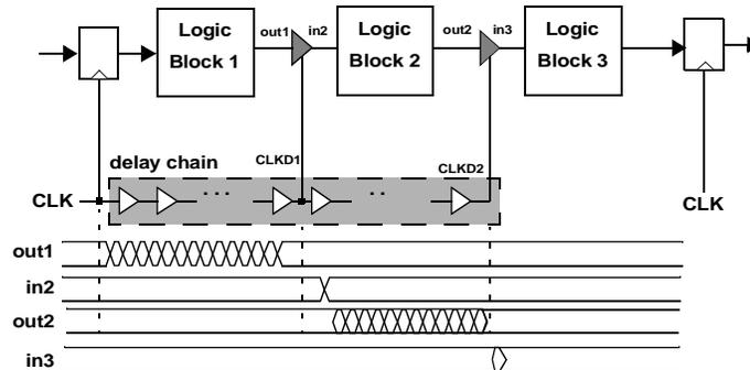
Figure 10.46 Application of self-timing for glitch reduction.
