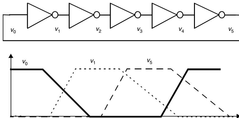
**Figure 1.20** Ring oscillator circuit for propagation-delay measurement.
