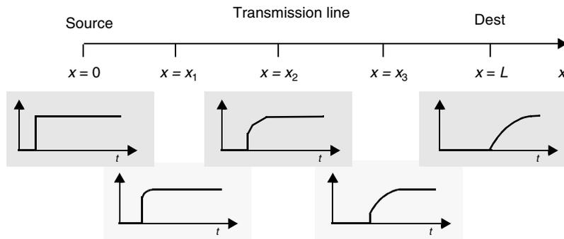
Figure 4.25 Step response of lossy transmission line.
