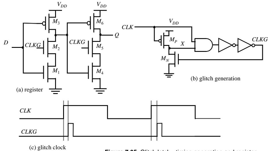
Figure 7.35 Glitch latch - timing generation and register.
