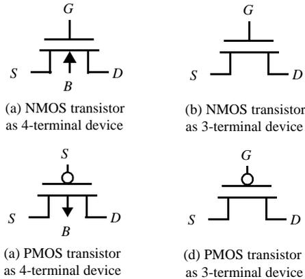
Figure 3.12 Circuit symbols for MOS transistors.
