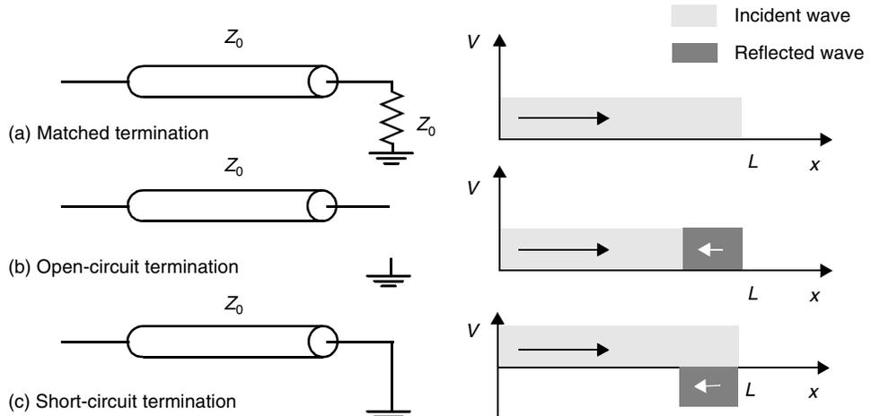
**Figure 4.19** Behavior of various transmission line terminations.
