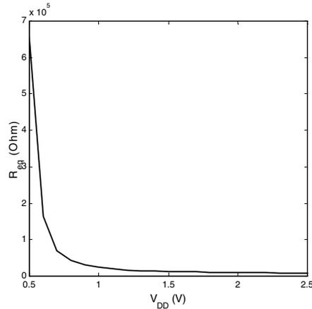
**Figure 3.27** Simulated equivalent resistance of a minimum size NMOS transistor in 0.25  $\mu\text{m}$  CMOS process as a function of  $V_{DD}$  ( $V_{GS} = V_{DD}$ ,  $V_{DS} = V_{DD} \rightarrow V_{DD}/2$ ).
