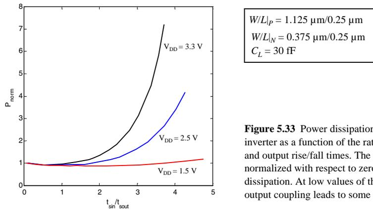
**Figure 5.33** Power dissipation of a static CMOS inverter as a function of the ratio between input and output rise/fall times. The power is normalized with respect to zero input rise-time dissipation. At low values of the slope ratio, input-output coupling leads to some extra dissipation.
