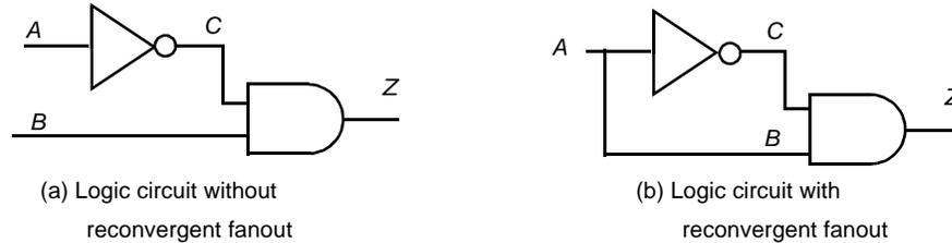
Figure 6.21 Example illustrating the effect of signal correlations.
