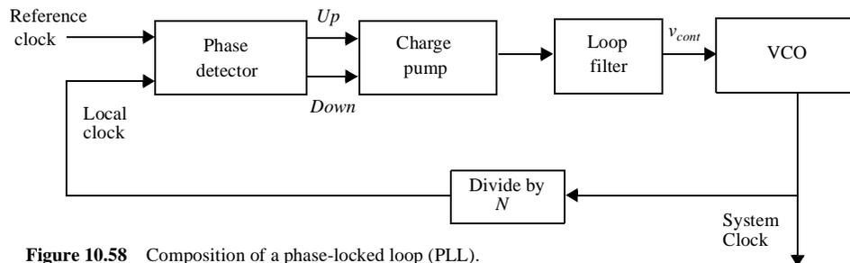
Figure 10.58 Composition of a phase-locked loop (PLL).
