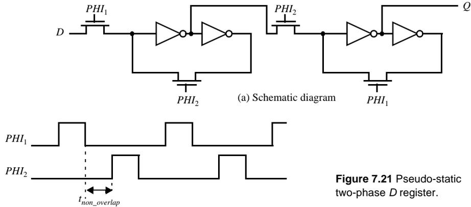
Figure 7.21 Pseudo-static two-phase  $D$  register.
