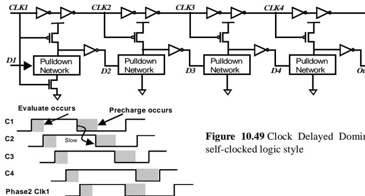
**Figure 10.49** Clock Delayed Domino Logic. A self-clocked logic style
