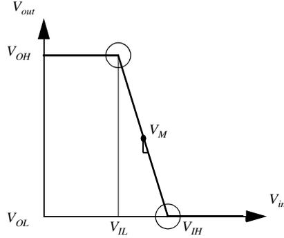
**Figure 5.9** A piece-wise linear approximation of the VTC simplifies the derivation of  $V_{IL}$  and  $V_{IH}$ .
