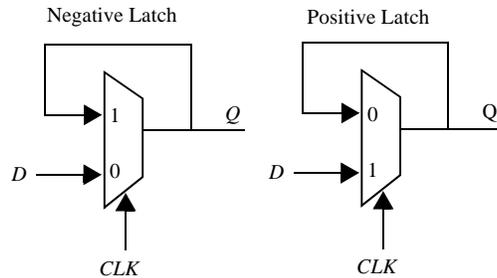
**Figure 7.11** Negative and positive latches based on multiplexers.
