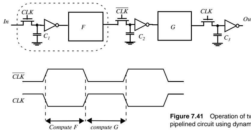
**Figure 7.41** Operation of two-phase pipelined circuit using dynamic registers.
