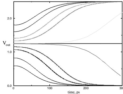
Figure 10.52 Simulated trajectory for a simple *flip-flop* synchronizer.
