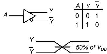
Figure 6.7 Differential Buffer.
