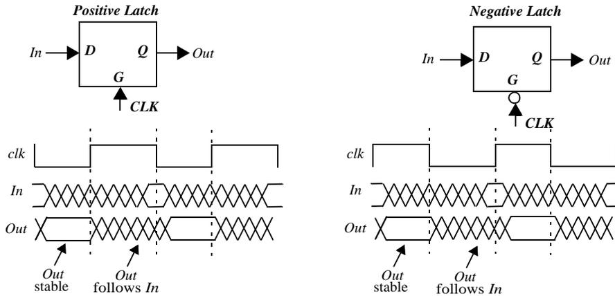
Figure 7.3 Timing of positive and negative latches.
