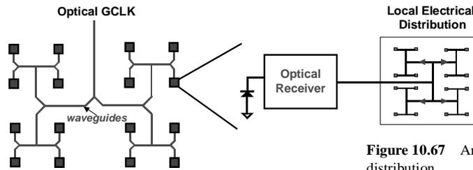
**Figure 10.67** Architecture for optical clock distribution.
