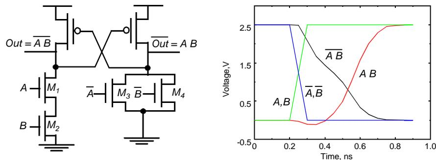
**Figure 6.31** Transient response of a simple AND/NAND DCVSL gate.  $M_1$  and  $M_2$   $1\mu\text{m}/0.25\mu\text{m}$ ,  $M_3$  and  $M_4$  are  $0.5\mu\text{m}/0.25\mu\text{m}$  and the cross-coupled PMOS devices are  $1.5\mu\text{m}/0.25\mu\text{m}$ .
