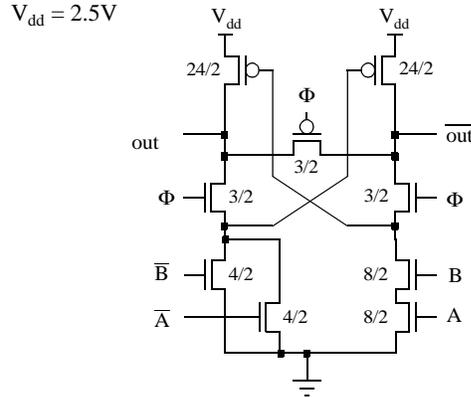
Figure 0.16 b - 2-input And Gate in SODS Style
