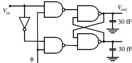
Figure 0.12 Simple synchronizer
