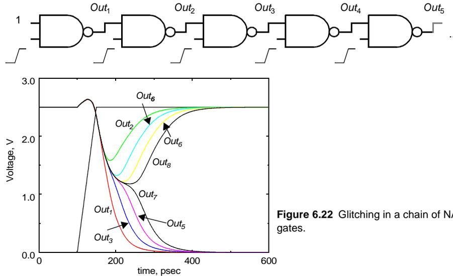
**Figure 6.22** Glitching in a chain of NAND gates.
