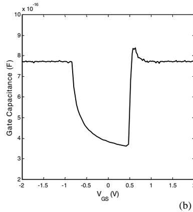
**Figure 3.31** Simulating the gate capacitance of an MOS transistor; (a) circuit configuration used for the analysis, (b) resulting capacitance plot for minimum-size NMOS transistor in 0.25  $\mu\text{m}$  technology.
