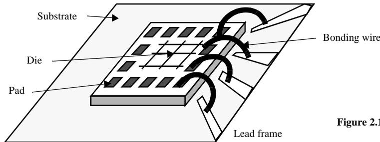
**Figure 2.11** Wire bonding.
