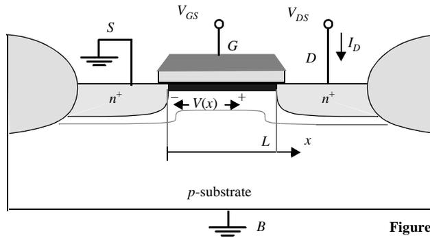
Figure 3.15 NMOS transistor with bias voltages.
