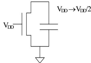
**Figure 0.13** The equivalent resistance is to be computed for the H→L transition.
