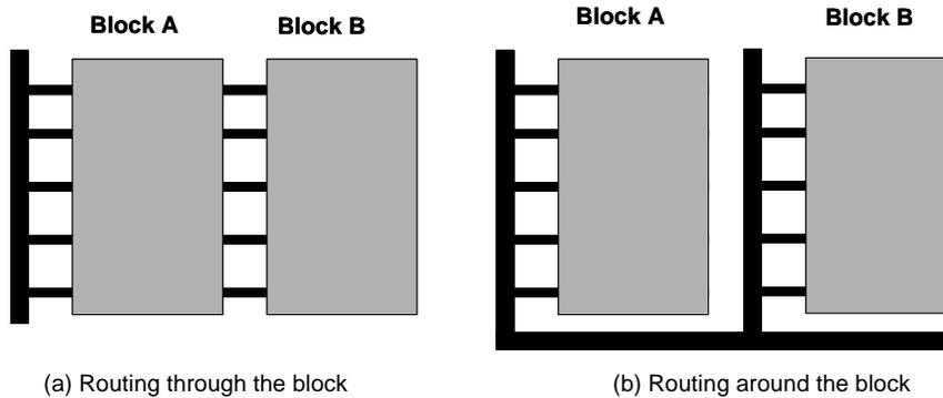
**Figure 1.8** Power distribution network design.
