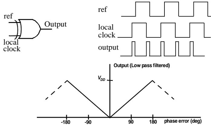
**Figure 10.59** The XOR as a phase detector.
