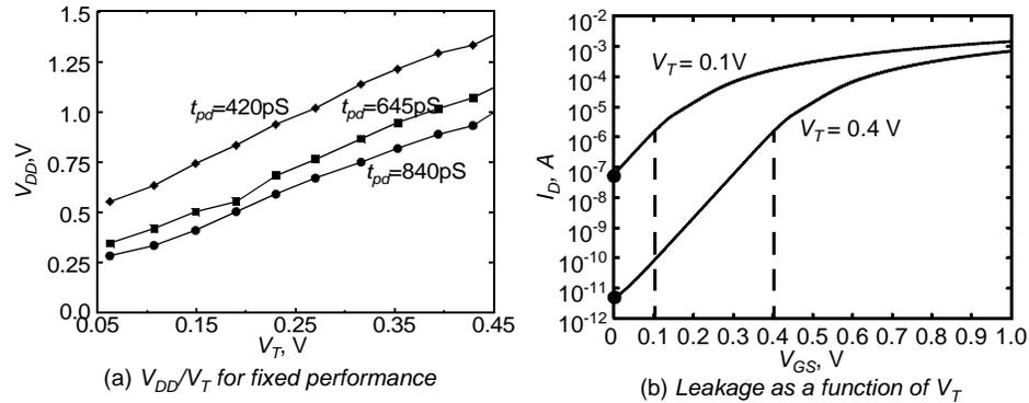
**Figure 6.72** Voltage Scaling ( $V_{DD}/V_T$  on delay and leakage)
