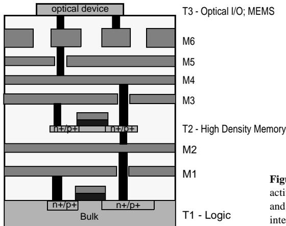
**Figure 2.20** Example of true 3D integration. Extra active layers (T\*), implementing high density memory and I/O, are sandwiched between the metal interconnect layers (M\*).
