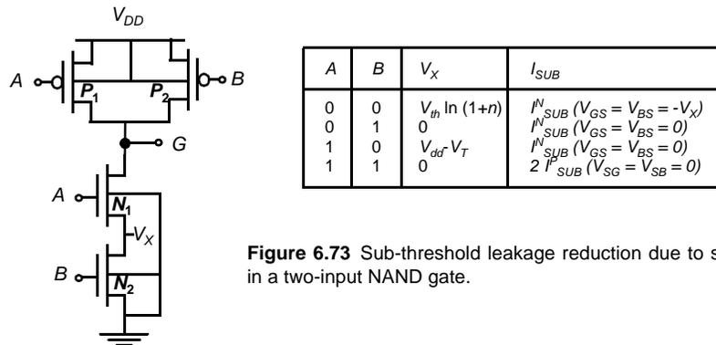
Figure 6.73 Sub-threshold leakage reduction due to stack effect in a two-input NAND gate.
