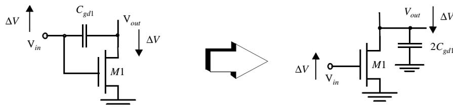
**Figure 5.14** The Miller effect—A capacitor experiencing identical but opposite voltage swings at both its terminals can be replaced by a capacitor to ground, whose value is two times the original value.
