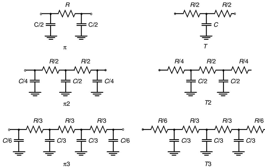
Figure 4.26 Simulation models for distributed  $RC$  line.
