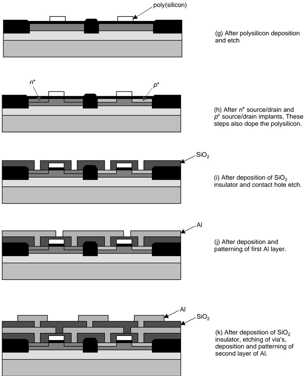
**Figure 2.7** Process flow for the fabrication of an NMOS and a PMOS transistor in a dual-well CMOS process. Be aware that the drawings are stylized for understanding, and that the aspects ratios are not proportioned to reality.
