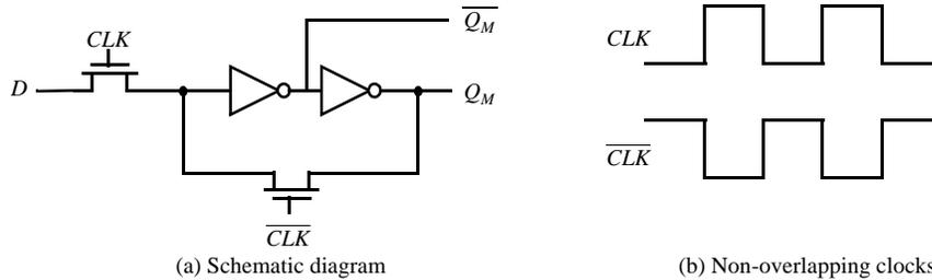
Figure 7.13 Multiplexer-based NMOS latch using NMOS-only pass transistors.
