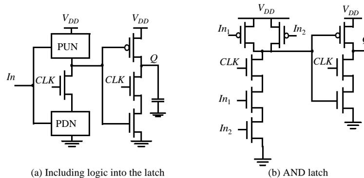
Figure 7.31 Adding logic to the TSPC approach.
