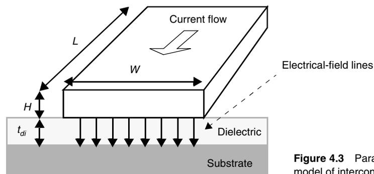
**Figure 4.3** Parallel-plate capacitance model of interconnect wire.
