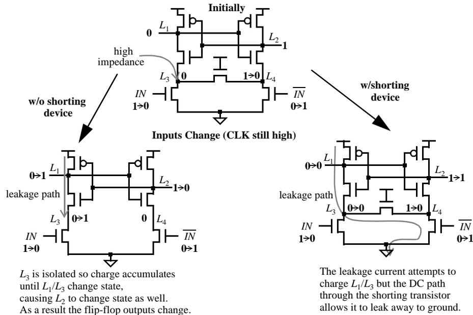
**Figure 7.39** The need for the shorting transistor  $M_4$ .
