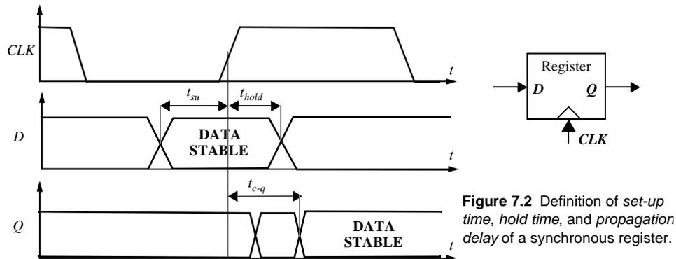
ing that the *set-up* and *hold*-times are met, the data at the  $D$  input is copied to the  $Q$  output after a worst-case *propagation delay* (with reference to the clock edge) denoted by  $t_{c-q}$ .
