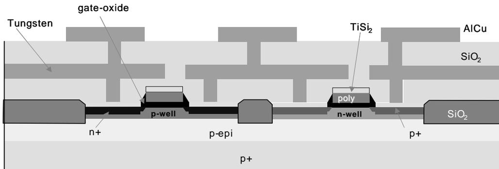
Figure 2.2 Cross section of modern dual-well CMOS process.
