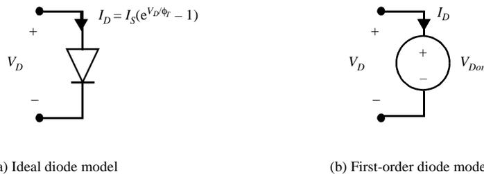
**Figure 3.6** Diode models.
