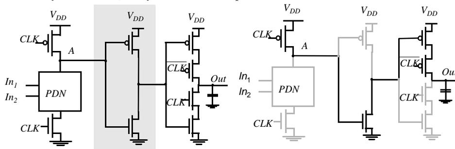
(a) Circuit with odd number of static inversions between dynamic logic stage and register
