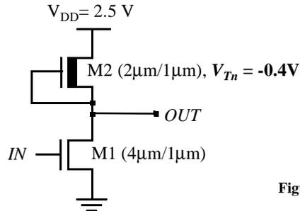
Figure 5.5 A depletion load NMOS inverter
