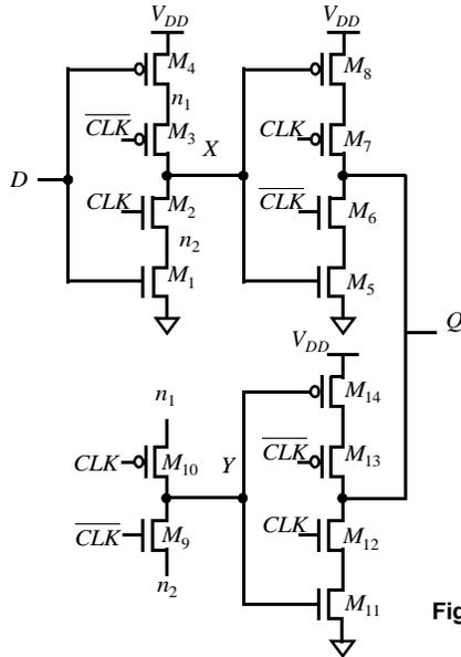
Figure 7.29 C<sup>2</sup>MOS based dual-edge triggered register.
