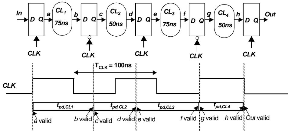
Figure 10.30 Latch-based pipeline.
