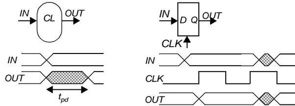
Figure 0.5 Timing diagrams of combinational logic and latch
