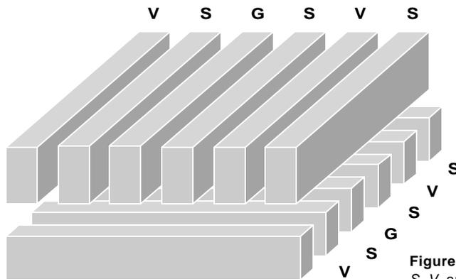
**Figure 9.6** Dense wire fabric (DWF) [Khatri99]. S, V, and G stand for Signal,  $V_{DD}$  and GND, respectively.
