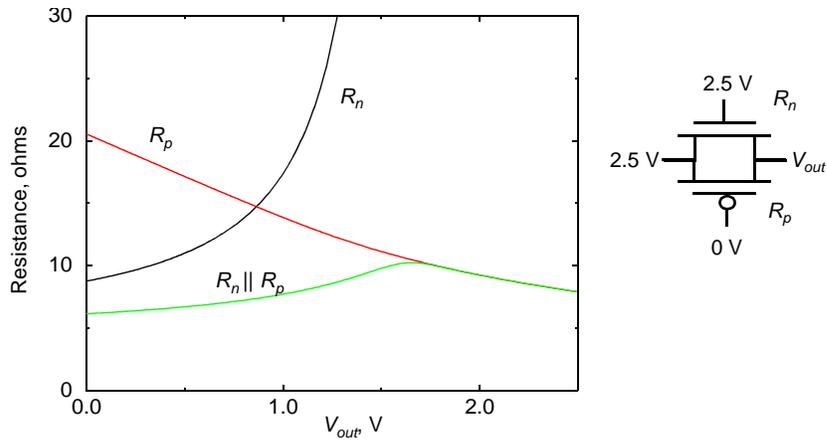
**Figure 6.48** Simulated equivalent resistance of transmission gate for low-to-high transition (for  $(W/L)_n = (W/L)_p = 0.5\mu\text{m}/0.25\mu\text{m}$ ). A similar response for overall resistance is obtained for the high-to-low transition
