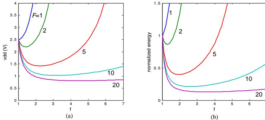
**Figure 5.29** Sizing of an inverter for energy-minimization. (a) Required supply voltage as a function of the sizing factor  $f$  for different values of the overall effective fanout  $F$ ; (b) Energy of scaled circuit (normalized with respect to the reference case) as a function of  $f$ .  $V_{ref} = 2.5V$ ,  $V_{TE} = 0.5V$ .
