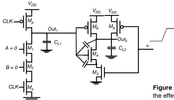
**Figure 6.62** Example demonstrating the effect of backgate coupling.
