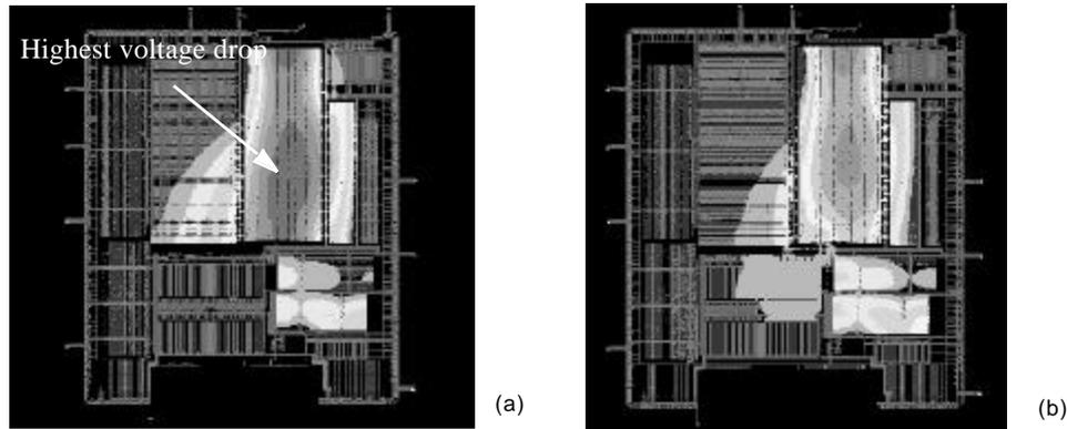
**Figure 9.15** Simulated IR voltage drop in power-distribution network of two versions of a complex digital integrated circuit. The gray-scale is used to indicate the severeness of the voltage drop. Adding an extra strap to the upper layers of the power network (b) helps to address the large voltage drop in the upper right module in the initial design (a).
