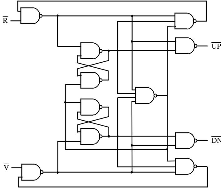
Figure 0.13 Phase-frequency comparator
