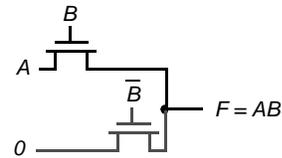
**Figure 6.33** Pass-transistor implementation of an AND gate.
