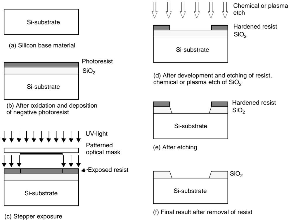
**Figure 2.5** Process steps for patterning of  $\text{SiO}_2$ .
