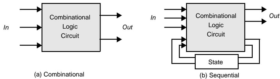
Figure 6.1 High level classification of logic circuits.
