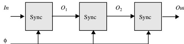
Figure 10.54 Cascading synchronizers reduces the main time-to-failure.
