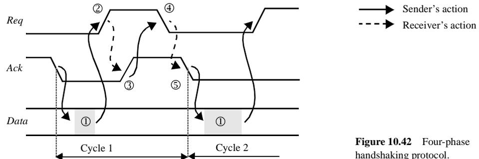
**Figure 10.42** Four-phase handshaking protocol.
