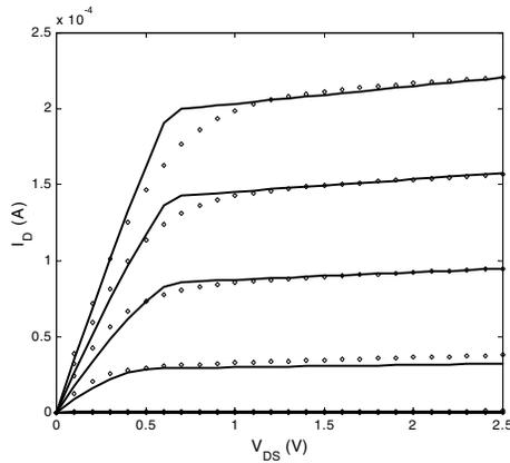
**Figure 3.24** Correspondence between simple model (solid line) and SPICE simulation (dotted) for minimum-size NMOS transistor ( $W_d=0.375 \mu\text{m}$ ,  $L_d=0.25 \mu\text{m}$ ). Observe the discrepancy in the transition zone between resistive and velocity saturation.
