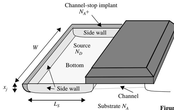
**Figure 3.32** Detailed view of source junction.
