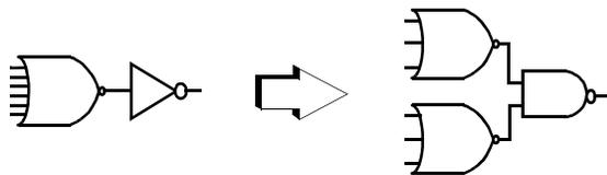
**Figure 6.16** Logic restructuring can reduce the gate fan-in.
