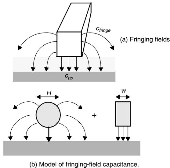
**Figure 4.4** The fringing-field capacitance. The model decomposes the capacitance into two contributions: a parallel-plate capacitance, and a fringing capacitance, modeled by a cylindrical wire with a diameter equal to the thickness of the wire.
