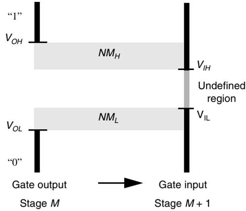
**Figure 1.13** Cascaded inverter gates: definition of noise margins.
