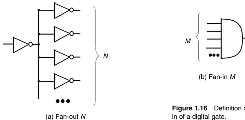
**Figure 1.16** Definition of fan-out and fan-in of a digital gate.
