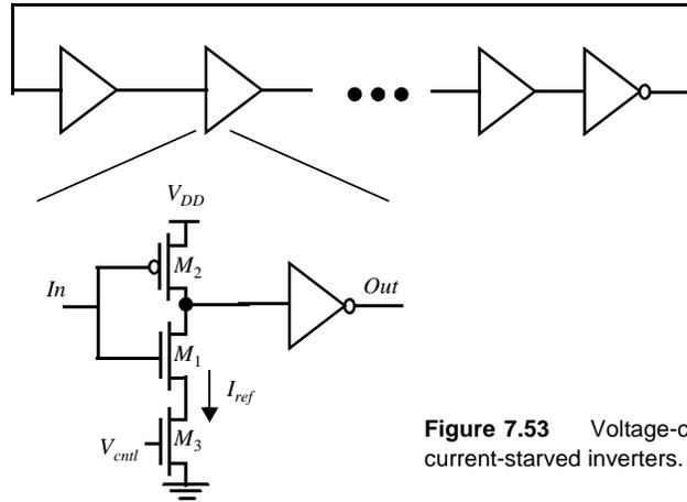
**Figure 7.53** Voltage-controlled oscillator based on current-starved inverters.
