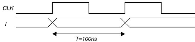
Figure 0.6 Input timing
