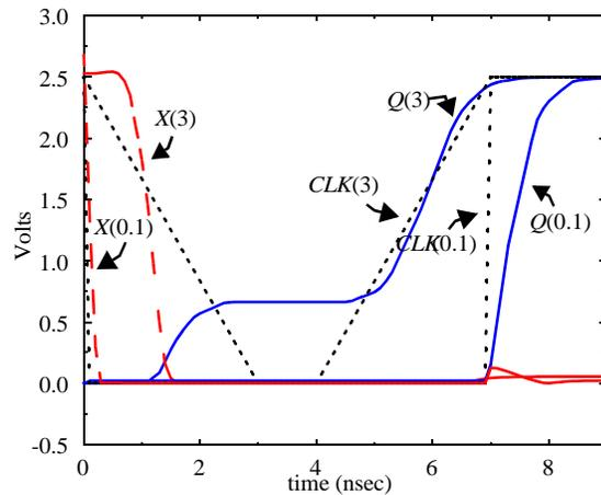
**Figure 7.28** Transient response of C<sup>2</sup>MOS FF for 0.1 nsec and 3 nsec clock rise (fall) times assuming  $ln = 1$ .
