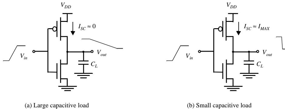
**Figure 5.31** Impact of load capacitance on short-circuit current.
