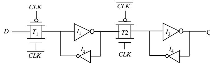
Figure 7.18 Reduced load clock load static *master-slave* register.
