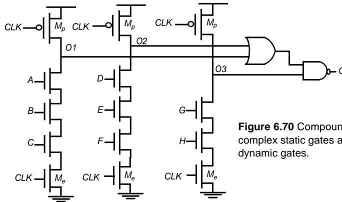
**Figure 6.70** Compound Domino logic uses complex static gates at the output of the dynamic gates.
