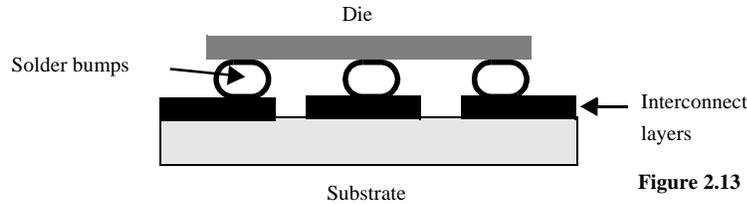
Figure 2.13 Flip-chip bonding.
