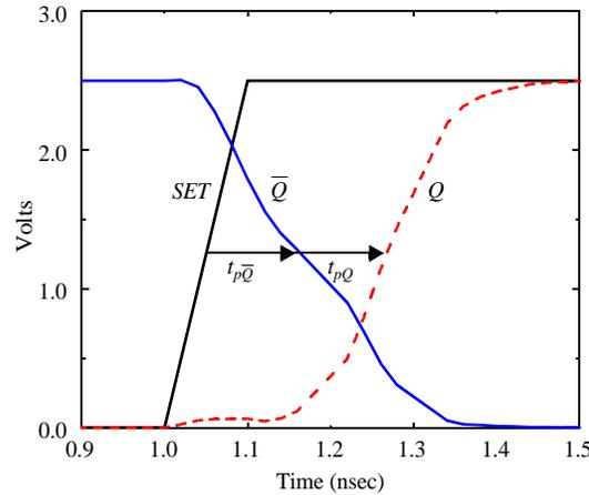
Figure 7.10 Transient response of SR flip-flop.
