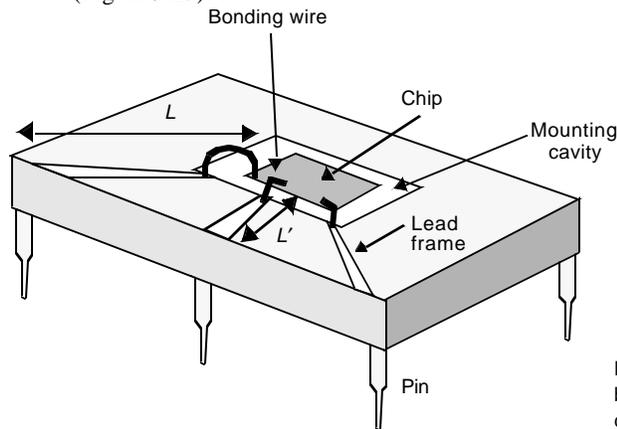
**Figure 9.23** The inductance of a bonding-wire/pin combination depends upon the pin position.
