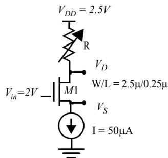
**Figure 0.4** Test configuration for the NMOS device.
