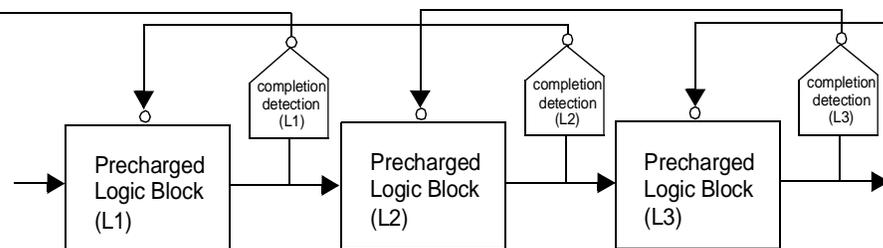
Figure 10.47 Self-resetting logic.
