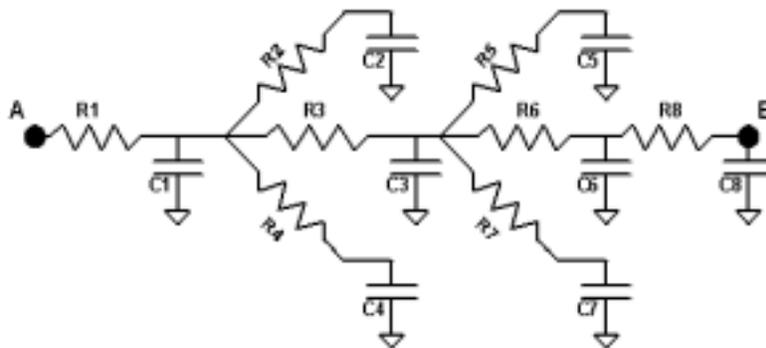
**Figure 0.4** RC tree for calculating the delay
