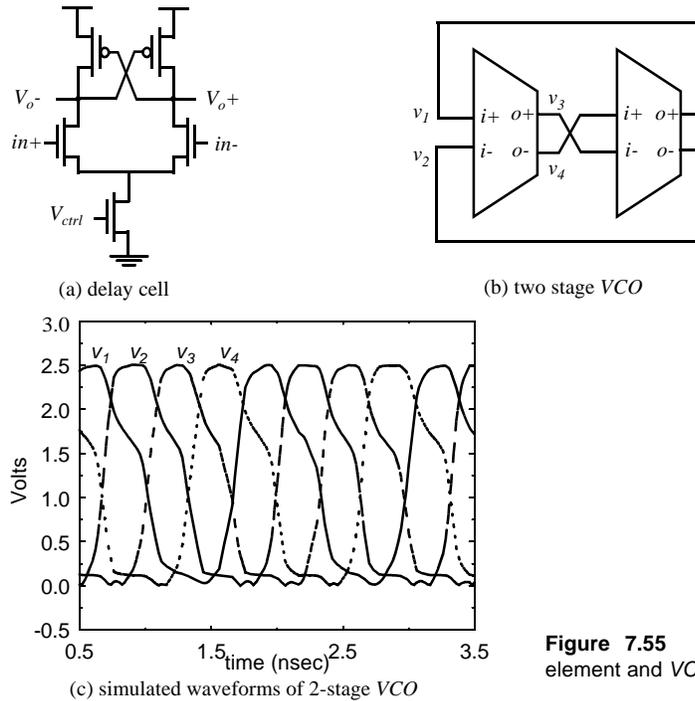
Figure 7.55 Differential delay element and VCO topology.
