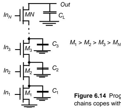
**Figure 6.14** Progressive sizing of transistors in large transistor chains copes with the extra load of internal capacitances.
