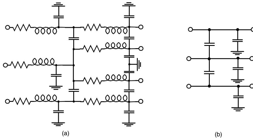
**Figure 4.2** Wire models for the circuit of Figure 4.1. Model (a) considers most of the wire parasitics (with the exception of inter-wire resistance and mutual inductance), while model (b) only considers capacitance.
