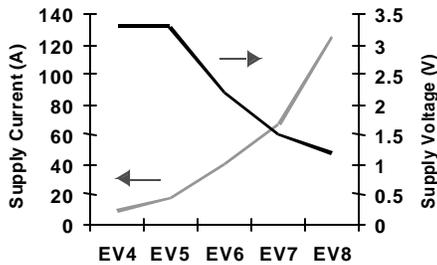
**Figure 9.12** Evolution of power-supply current and supply voltage for different generations of the high-performance alpha microprocessor family from Compaq. Even with the reductions in supply voltage, a total supply current of over 100 A has to be supported for the newer generations.
