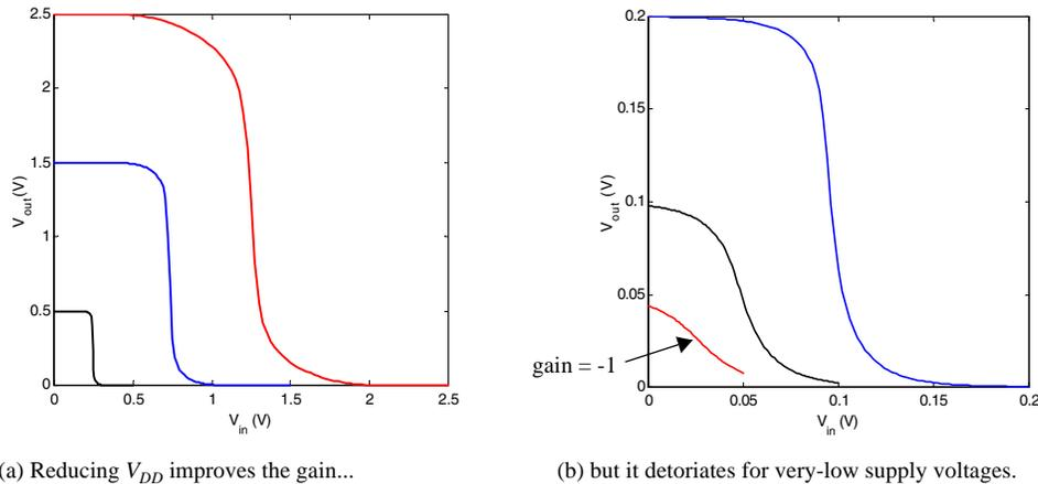
(a) Reducing  $V_{DD}$  improves the gain...
