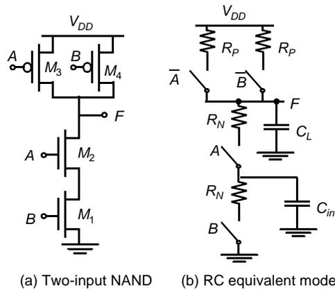
**Figure 6.8** Equivalent RC model for a 2-input NAND gate.
