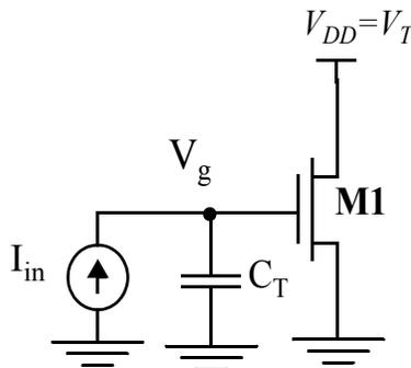
**Figure 0.14** Circuit to measure total input capacitance
