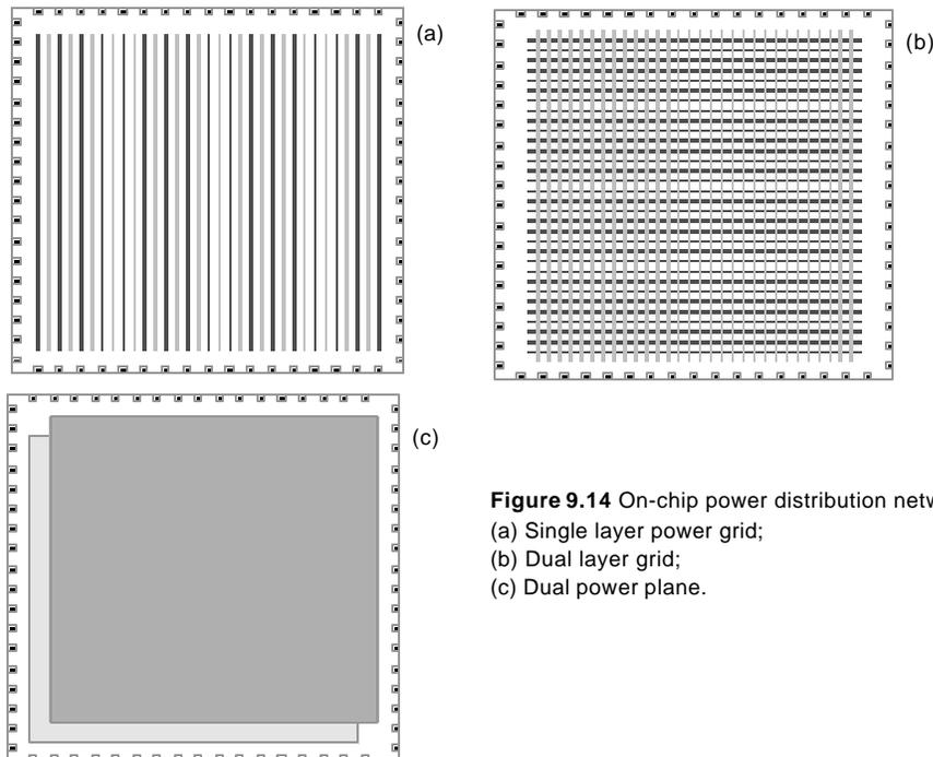
**Figure 9.14** On-chip power distribution networks.
