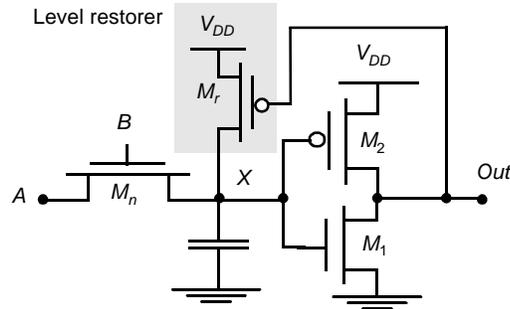
Figure 6.39 Level-restoring circuit.
