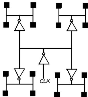
**Figure 10.18** Example of an *H-tree* clock-distribution network for 16 leaf nodes.
