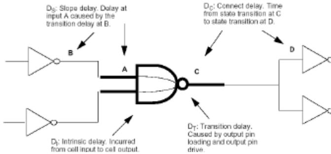
Figure E.1 Delay components.
