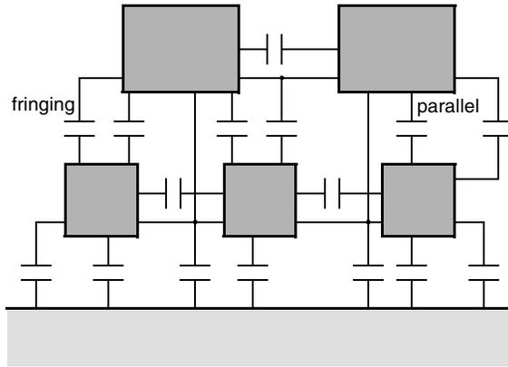
**Figure 4.6** Capacitive coupling between wires in interconnect hierarchy.
