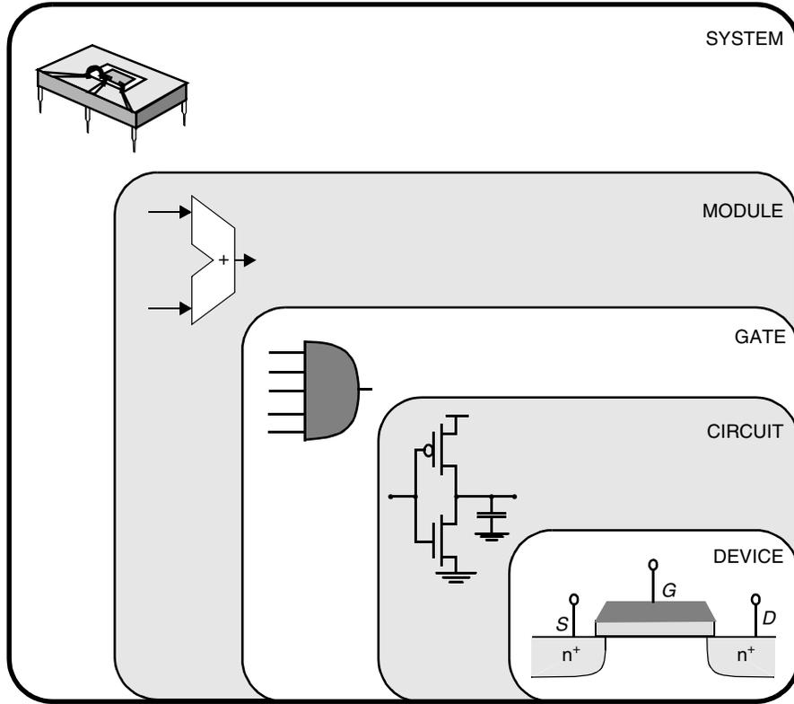
**Figure 1.6** Design abstraction levels in digital circuits.
