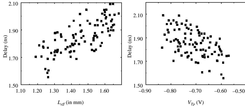
**Figure 3.38** Distribution plots of speed of adder circuit as a function of varying device parameters, as obtained by a Monte Carlo analysis. The circuit is implemented in a 2  $\mu\text{m}$  (nominal) CMOS technology (courtesy of Eric Boskin, UCB, and ATMEL corp.).
