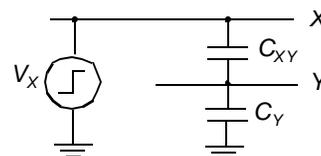
**Figure 9.1** Capacitive coupling to a floating line.
