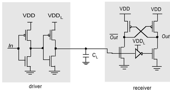
**Figure 9.31** Single-ended, static reduced-swing driver and receiver.
