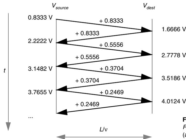
**Figure 4.22** Lattice diagram for  $R_S = 5Z_0$  and  $R_L = \infty$ ,  $V_{step} = 5$  V, (as in Figure 4.21a).
