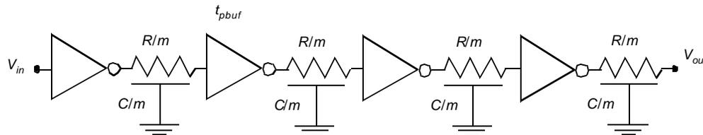
**Figure 9.19** Reducing RC interconnect delay by introducing repeaters.
