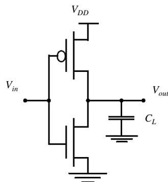
**Figure 5.1** Static CMOS inverter.  $V_{DD}$  stands for the supply voltage.
