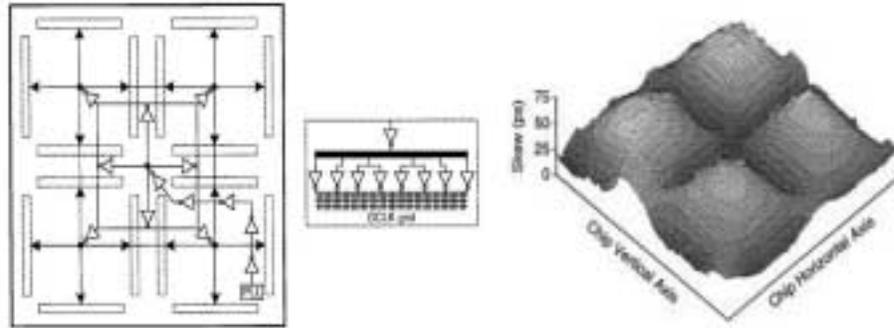
**Figure 10.25** Global clock-distribution network in a window-pane structure.
