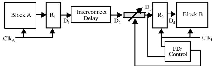
**Figure 10.2** Mesochronous communication approach using variable delay line.
