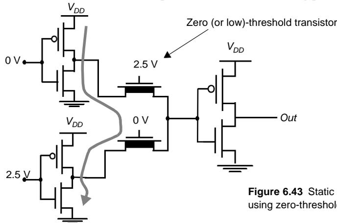
Figure 6.43 Static power consumption when using zero-threshold pass-transistors.
