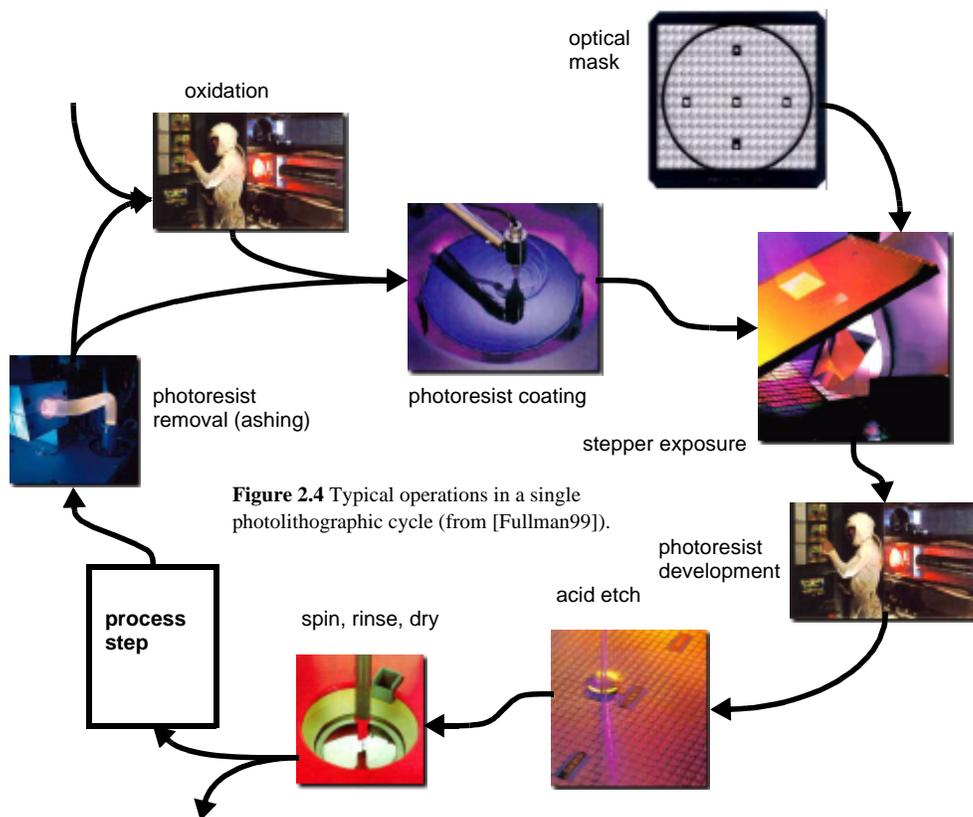
Figure 2.4 Typical operations in a single photolithographic cycle (from [Fullman99]).
