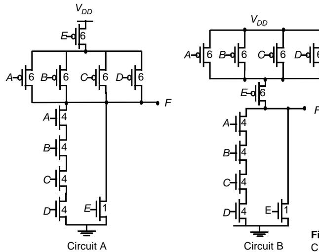
**Figure 6.2** Two static CMOS gates.
