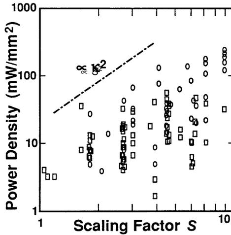
**Figure 5.40** Evolution of power-density in micro- and DSP processors, as a function of the scaling factor  $S$  ([Sakurai97]).  $S$  is normalized to 1 for a 4  $\mu\text{m}$  process.
