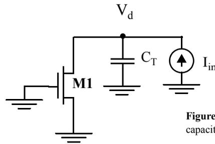
**Figure 0.15** Circuit to measure the total drain capacitance
