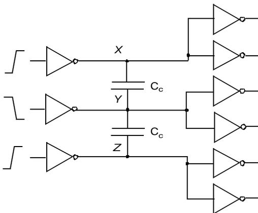
**Figure 9.5** Impact of cross talk on propagation delay.
