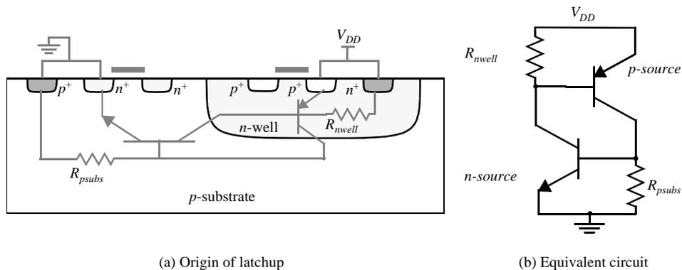
Figure 3.37 CMOS latchup.
