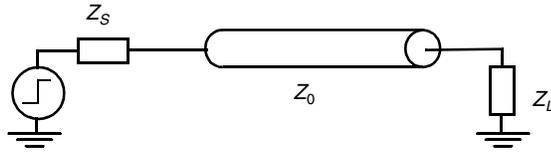
**Figure 4.20** Transmission line with terminating impedances.
