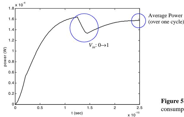
Figure 5.38 Deriving the power consumption using SPICE.
