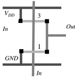
**Figure A.2** Sticks representation of CMOS inverter. The numbers represent the (*Width/Length*)-ratios of the transistors.
