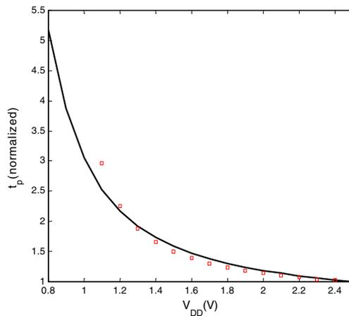
**Figure 5.17** Propagation delay of CMOS inverter as a function of supply voltage (normalized with respect to the delay at 2.5 V). The dots indicate the delay values predicted by Eq. (5.21). Observe that this equation is only valid when the devices are velocity-saturated. Hence, the deviation at low supply voltages.
