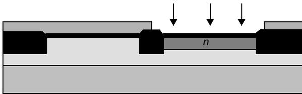
(e) After  $n$ -well and  $V_{Tp}$  adjust implants
