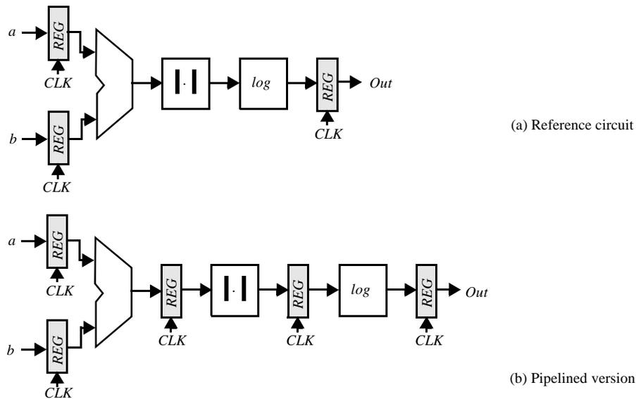
**Figure 7.40** Datapath for the computation of  $\log(|a + b|)$ .
