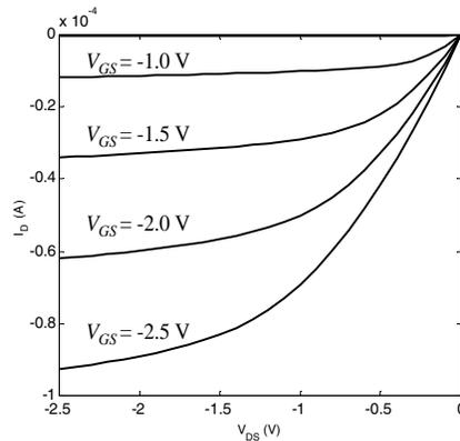
**Figure 3.21**  $I$ - $V$  characteristics of ( $W_d=0.375 \mu\text{m}$ ,  $L_d=0.25 \mu\text{m}$ ) PMOS transistor in 0.25  $\mu\text{m}$  CMOS process. Due to the smaller mobility, the maximum current is only 42% of what is achieved by a similar NMOS transistor.
