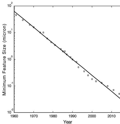
**Figure 3.39** Evolution of (average) minimum channel length of MOS transistors over time. Dots represent observed or projected (2000 and beyond) values. The continuous line represents a scaling scenario that reduces the minimum feature with a factor 2 every 5 years.
