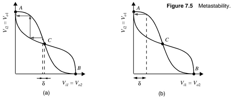
On the other hand,  $A$  and  $B$  are stable operation points, as demonstrated in Figure 7.5b. In these points, the **loop gain is much smaller than unity**. Even a rather large deviation from the operation point is reduced in size and disappears.
