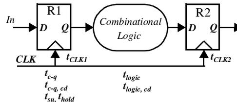
Figure 10.5 Pipelined Datapath Circuit and timing parameters.
