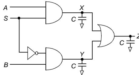
Figure 6.18 Two-input multiplexer
