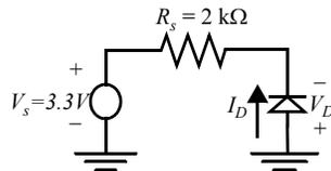
Figure 0.2 Series diode circuit
