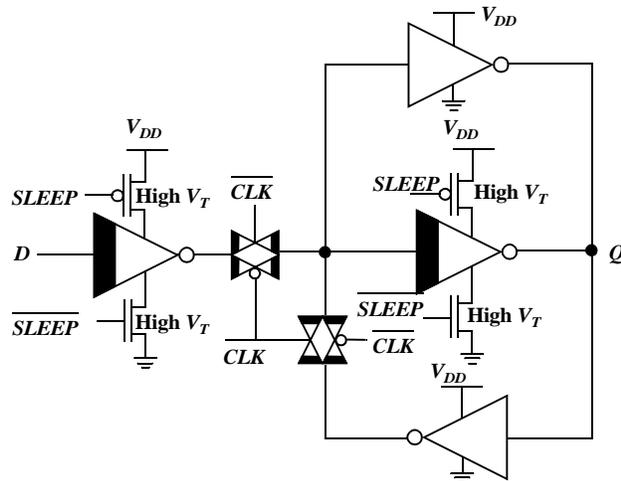
**Figure 7.23** Solving the leakage problem using multiple-threshold CMOS.
