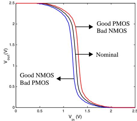
**Figure 5.11** Impact of device variations on static CMOS inverter VTC. The “good” device has a smaller oxide thickness (-3nm), a smaller length (-25 nm), a higher width (+30 nm), and a smaller threshold (-60 mV). The opposite is true for the “bad” transistor.
