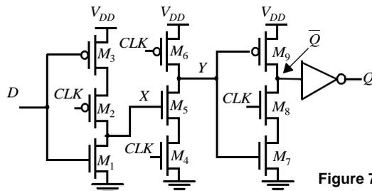
**Figure 7.33** Positive edge-triggered register TSPC.
