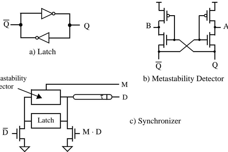
Figure 0.14 Simple synchronizer
