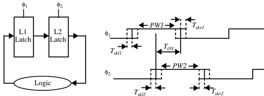
Figure 0.9 Timing constraints
