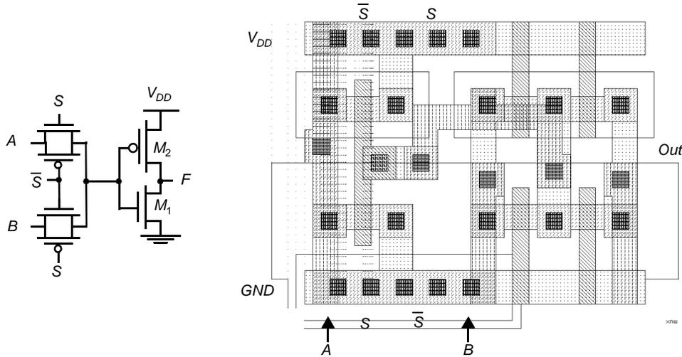
Figure 6.46 Transmission gate multiplexer and its layout.
