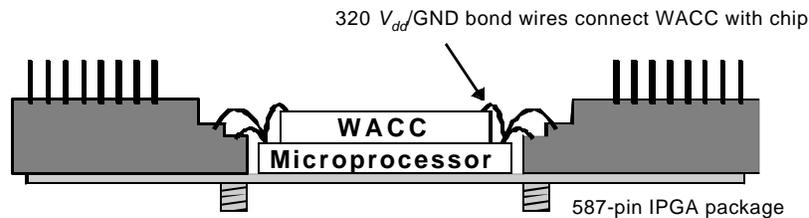
**Figure 9.25** The Wirebond-attached Chip capacitor (WACC) approach provides extra decoupling capacitance close to the chip for the Compaq EV6 microprocessor [Herrick00]. The microprocessor is connected to the outside world via 320 signal pins and 198 supply/ground pins.
