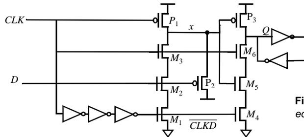
**Figure 7.36** Flow-through positive edge-triggered register.
