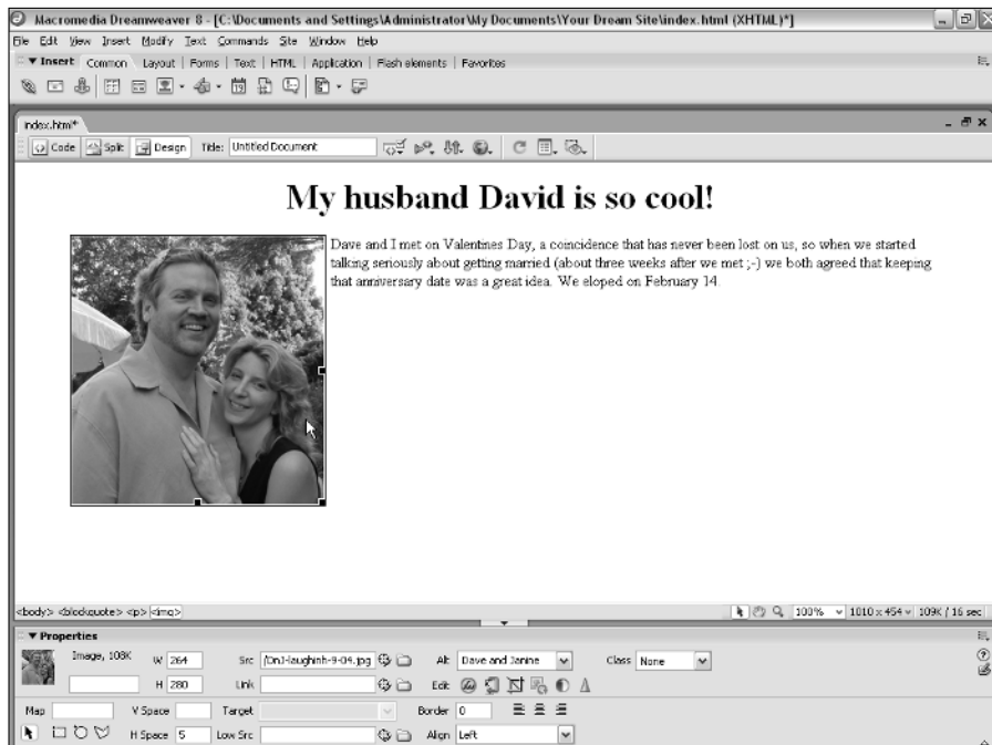
Figure 2-6: When an image is selected, the Properties inspector provides easy access to common image attributes, such as alignment and spacing.
