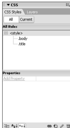
Figure 8-2: The new CSS panel, showing all the styles associated with the open document.
