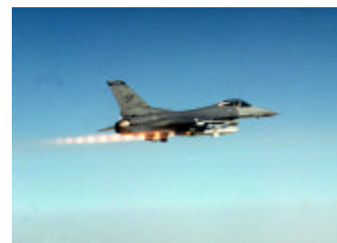
F-16CJ's use a high-speed antiradiation missile (HARM) targeting system and missiles to suppress or disable enemy radars.
