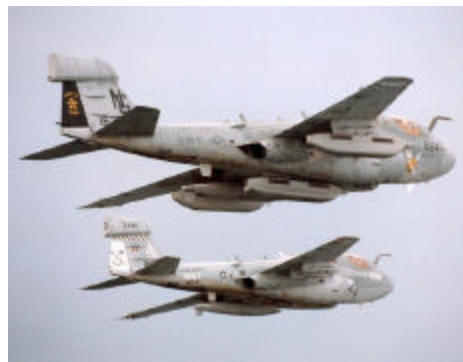
The EA-6B is a joint EW platform that can detect threats, provide standoff jamming, and can carry HARMs.
