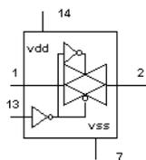
The 4066 device has four independent bilateral analogue switches (transmission gates). Each switch has two input/output terminals (Y/Z) and an active HIGH enable input (E).
