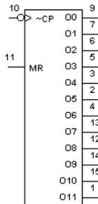
The 4040 device is a 12-stage binary ripple counter with a clock input (CP), an overriding asynchronous master reset input (MR) and twelve fully buffered outputs ( $O_0$  to  $O_{11}$ ).
