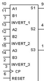
The 4038 triple serial adder has the clock and carry reset inputs common to all three adders. The carry is added on the negative-going clock transition for this device.
