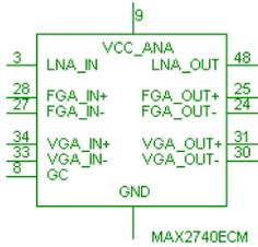
The MISC family contains footprint information for a number of components, for example, the Integrated GPS Receiver/Synthesizer shown here.
