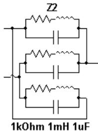
Z Load 1 Delta is a delta connection of three Z Load 1s as shown.
