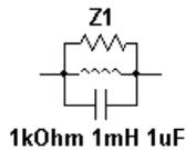
Z Load 3 is a circuit block with an RLC parallel connection with R, L and C values as shown.
