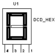
The seven-segment display actively shows its state while the circuit is running. The seven terminals (left to right, respectively) control segments a to g. By giving the proper binary-digit inputs to segments a to g, you can display decimal numbers from 0 to 9 and letters A to F.
