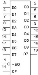
The 40374 device is an octal D-type flip-flop with 3-state buffered outputs with a common clock input (CP). It is used primarily as an 8-bit positive edge-triggered storage register for interfacing with a 3-state bus.
