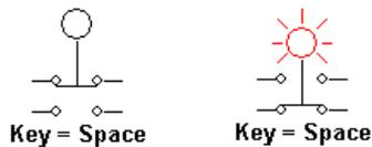
Press the switch's key during simulation to make the switch toggle positions.
