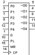
The 4018 device is a 5-stage Johnson counter with a clock input (CP), a data input (D), an asynchronous parallel load input (PL), five parallel inputs (P0 to P4), five active **LOW** buffered outputs ( $\overline{O0}$  to  $\overline{O4}$ ), and an overriding asynchronous master reset input ( $\overline{MR}$ ).
