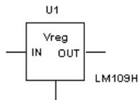
The linear IC voltage regulator is a device used to hold the output voltage from a dc power supply relatively constant over a wide range of line and load variations. Most commonly used IC voltage regulators are three-terminal devices.
