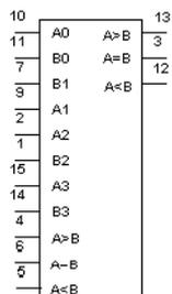
The 4585 device is a 4-bit magnitude comparator that compares two 4-bit words (A and B), whether they are “less than”, “equal to”, or “greater than”. Each word has four parallel inputs (A0 to A3 and B0 to B3).
