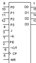
The 4035 device is a fully synchronous edge-triggered 4-bit shift register with a clock input (CP), four synchronous parallel data inputs (P0 to P3), two synchronous serial data inputs (J,  $\bar{K}$ ), a synchronous parallel enable input (PE), buffered parallel outputs from all 4-bit positions (O0 to O3), a true/complement input ( $T/\bar{C}$ ) and an overriding asynchronous master reset input (MR).
