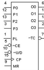
This binary up/down counter counts from 0000 to 1111 in binary (0 to 15 in decimal).
