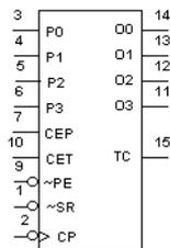
The 40163 device is a fully synchronous edge-triggered 4-bit binary counter with a clock input (CP), four synchronous parallel data inputs (P0 to P3), four synchronous mode control inputs (parallel enable ( $\overline{\text{PE}}$ ), count enable parallel (CEP) and count enable trickle (CET)), and synchronous reset ( $\overline{\text{SR}}$ ), buffered outputs from all four bit positions (O0 to O3) and a terminal count output (TC).
