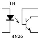
An optocoupler is a device that uses light to couple a signal from its input (a photoemitter) to its output (a photodetector).
