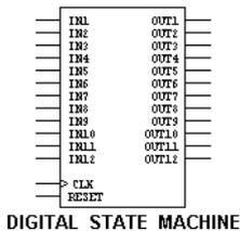
The digital state machine's model can be configured to act as most types of counter or clocked combinational logic blocks. Use this device to replace large digital schematics.
