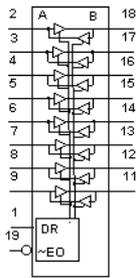
The 40245 device, an octal bus transmitter/receiver with 3-state outputs, is designed for 8-line asynchronous, 2-way data communication between data buses.
