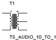
The transformer is one of the most common and useful applications of inductance. It can step up or step down an input primary voltage ( $V_1$ ) to a secondary voltage ( $V_2$ ). The relationship is given by  $V_1/V_2 = n$ , where  $n$  is the ratio of the primary turns to the secondary turns. The parameter  $n$  can be adjusted by editing the transformer's model.
