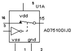
This switch is a resistor that varies logarithmically between specified values of a controlling input voltage. Note that the input is not internally limited. Therefore, if the controlling signal exceeds the specified Coff or Con values, the resistance may become excessively large or small.
