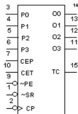
The 40162 device is a fully synchronous edge-triggered 4-bit decade counter with a clock input (CP), four synchronous parallel data inputs (P0 to P3), four synchronous mode control inputs (parallel enable ( $\overline{\text{PE}}$ ), count enable parallel (CEP) and count enable trickle (CET)), and synchronous reset ( $\overline{\text{SR}}$ ), buffered outputs from all four bit positions (O0 to O3) and a terminal count output (TC).
