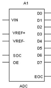
An ADC is a special type of encoder that converts the input analog voltage to an equivalent output digital word.
