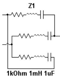
Z Load 2 Delta is a delta connection of three Z Load 2s as shown.
