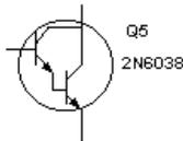
The Darlington connection is a pair of two bipolar junction transistors for operation as a composite transistor. The composite transistor acts as a single unit with a current gain that is the product of the current gains of each bipolar junction transistor.
