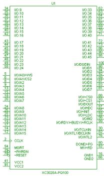
A number of FPGAs (Field Programmable Gate Arrays) are included that have symbols for layout purposes. These also have footprint, but no model information.
