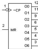
The 4024 is a 7-stage binary ripple counter. A high on MR (Master Reset) forces all counter stages and outputs low.
