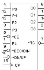
The 4029 is a synchronous edge-triggered up/down 4-bit binary/BCD decade counter with a clock input (CP), an active LOW count enable input ( $\overline{CE}$ ), an up/down control input (UP/ $\overline{DN}$ ), a binary/decade control input (BIN/ $\overline{DEC}$ ), an overriding asynchronous active HIGH parallel load input (PL), four parallel data inputs (P0 to P3), four parallel buffered outputs (O0 to O3) and an active LOW terminal count output ( $\overline{TC}$ ).
