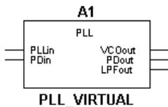
This component models the behavior of a phase-locked loop circuit, which is a circuit that contains an oscillator whose output phase and frequency are steered to keep it synchronized with an input reference signal.
