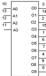
The 4028 device is a 4-bit BCD to 1-of-10 active HIGH decoder.
