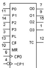
The 4526 device is a synchronous programmable 4-bit binary down counter with an active HIGH and an active LOW clock input (CP0,  $\overline{CP1}$ ), an asynchronous parallel load input (PL), four parallel inputs (P0 to P3), a cascade feedback input (CF), four buffered parallel outputs (O0 to O3), a terminal count output (TC) and an overriding asynchronous master reset input (MR).
