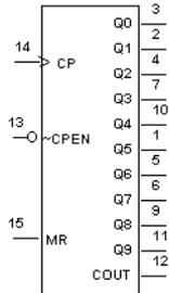
The 4017 device is a 5-stage Johnson decade counter with ten spike-free decoded active HIGH outputs ( $O_0$  to  $O_9$ ), an active LOW output from the most significant flip-flop ( $\overline{O}_{5,9}$ ), active HIGH and active LOW clock inputs ( $CP_0$ ,  $\overline{CP}_1$ ) and an overriding asynchronous master reset input (MR).
