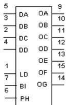
The 4543 device is a BCD to 7-segment latch/decoder/driver for liquid crystal and LED displays. It has four address inputs (DA to DD), an active HIGH latch disable input (LD), an active HIGH blanking input (BI), an active HIGH phase input (PH) and seven buffered segment outputs (Oa to Og).
