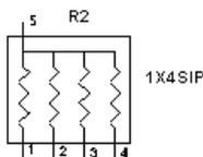
Resistor packs are collections of resistors within a single package. The configuration of the resistors can be varied based on the intended usage of the package. Resistor packs are used to minimize the amount of space required on the PCB for the design. In some applications, noise can be a consideration for the use of resistor packs.
