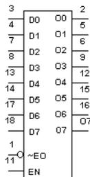
The 40373 device is an 8-bit transparent latch with 3-state buffered outputs.
