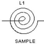
From many types of RF inductors, spiral inductors provide higher inductance values and higher  $Q$ s. The spiral inductor is a technique of forming a planar inductor in a small place. The shape is described by an increasing radius with angle: i.e.  $R = r/I + k\theta$
