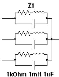
Z Load 1 Wye is a delta connection of three Z Load 1s as shown.
