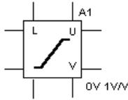
A voltage “clipper”. This component is a single input, single output function. The output is restricted to the range specified by the output lower and upper limits. Output smoothing occurs within the specified range. The voltage-controlled limiter will operate in DC, AC and transient analysis modes.
