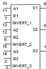
The 4032 triple serial adder has the clock and carry reset inputs common to all three adders. The carry is added on the positive-going clock transition for this device.
