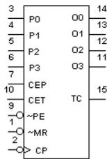
The 40161 device is a fully synchronous edge-triggered 4-bit binary counter with a clock input (CP), an overriding asynchronous master reset ( $\overline{\text{MR}}$ ), four parallel data inputs (P0 to P3), three synchronous mode control inputs (parallel enable ( $\overline{\text{PE}}$ ), count enable parallel (CEP) and count enable trickle (CET)), buffered outputs from all four bit positions (O0 to O3) and a terminal count output (TC).
