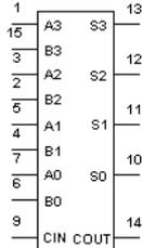
This device is capable of adding two 4-bit binary numbers together.
