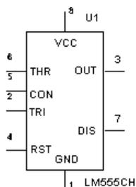
The 555 timer is an IC chip that is commonly used as an astable multivibrator, a monostable multivibrator or a voltage-controlled oscillator. The 555 timer consists basically of two comparators, a resistive voltage divider, a flip-flop and a discharge transistor. It is a two-state device whose output voltage level can be either high or low. The state of the output can be controlled by proper input signals and time-delay elements connected externally to the 555 timer.
