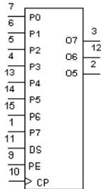
The 4014 device is a fully synchronous edge-triggered 8-bit static shift register with eight synchronous parallel inputs ( $P_0$  to  $P_7$ ), a synchronous serial data input ( $D_S$ ), a synchronous parallel enable input (PE), a LOW to HIGH edge-triggered clock input (CP) and buffered parallel outputs from the last three stages ( $O_5$  to  $O_7$ ).
