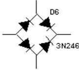
The full-wave bridge rectifier uses four diodes to perform full-wave rectification of an input AC voltage. Two diodes conduct during each half cycle, giving a full-wave rectified output voltage. The top and bottom terminals can be used as the input terminals for the AC voltage. The left and right terminals can be used as the output DC terminals.
