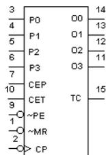
The 40160 device is a fully synchronous edge-triggered 4-bit decade counter with a clock input (CP), an overriding asynchronous master reset ( $\overline{\text{MR}}$ ), four parallel data inputs (P0 to P3), three synchronous mode control inputs (parallel enable ( $\overline{\text{PE}}$ ), count enable parallel (CEP) and count enable trickle (CET)), buffered outputs from all four bit positions (O0 to O3) and a terminal count output (TC).
