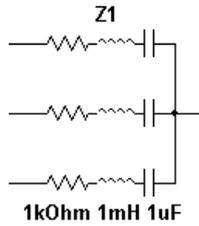
Z Load 2 Wye is a wye connection of three Z Load 2s as shown.
