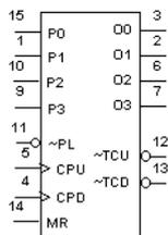
The 40193 device is a 4-bit synchronous up/down binary counter with a count-up clock input (CPU), a count-down clock input (CPD), an asynchronous parallel load input ( $\overline{PL}$ ), four parallel data inputs (P0 to P3), an asynchronous master reset input (MR), four counter outputs (O0 to O3), an active LOW terminal count-up (carry) output ( $\overline{TCU}$ ) and an active LOW terminal count-down (borrow) output ( $\overline{TCD}$ ).
