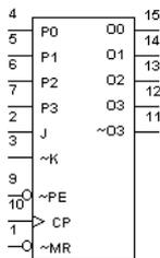
The 40195 device is a fully synchronous edge-triggered 4-bit shift register with a clock input (CP), four synchronous parallel data inputs (P0 to P3), two synchronous serial data inputs (J,  $\overline{K}$ ), a synchronous parallel enable input ( $\overline{PE}$ ), buffered parallel outputs from all 4-bit positions (O0 to O3), a buffered inverted output from the last bit position ( $\overline{O3}$ ) and an overriding asynchronous master reset input ( $\overline{MR}$ ).
