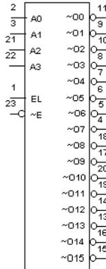
This device is a 1-of-16 decoder/demultiplexer with input latches. The input latches allow for the user to hold a previous input with the enable input while the inputs change.
