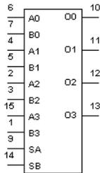
The 4519 device provides four multiplexing circuits with common select inputs (SA, SB). Each circuit contains two inputs (An, Bn) and one output (On).
