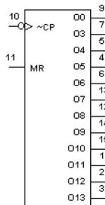
The 4020 device is a 14-stage binary ripple counter with a clock input ( $\overline{CP}$ ), an overriding asynchronous master reset input (MR) and twelve fully buffered outputs (O<sub>0</sub>, O<sub>3</sub> to O<sub>13</sub>).
