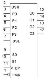
The 40194 device is a 4-bit bidirectional shift register with two mode control inputs (S0 and S1), a clock input (CP), a serial data shift left input (DSL), a serial data shift right input (DSR), four parallel data inputs (P0 to P3), an overriding asynchronous master reset input ( $\overline{\text{MR}}$ ), and four buffered parallel outputs (O0 to O3).
