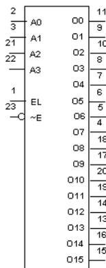
This device is a 1-of-16 decoder/demultiplexer with input latches. The input latches allow for the user to hold a previous input with the enable input while the inputs change.
