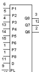
The 4021 device is an 8-bit static shift register (parallel-to-serial converter) with a synchronous serial data input ( $D_8$ ), a clock input (CP), an asynchronous active HIGH parallel load input (PL), eight asynchronous parallel data inputs ( $P_0$  to  $P_7$ ) and buffered parallel outputs from the last three stages ( $O_5$  to  $O_7$ ).
