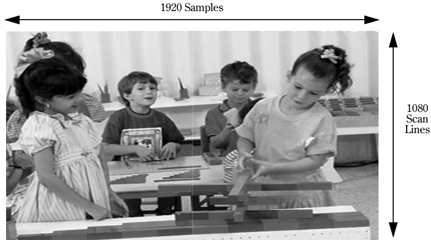
Figure 7.38. Scaling 4:3 Content for a 16:9 Display: “Panorama” mode. Left and right 25% edges of picture are nonlinearly scaled horizontally to fill 16:9 display, distorted picture on left and right sides.
