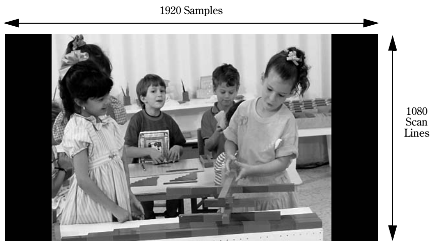
Figure 7.35. Scaling 4:3 Content for a 16:9 Display: "Normal" mode. Left and right portions of 16:9 display not used, so made black or gray.
