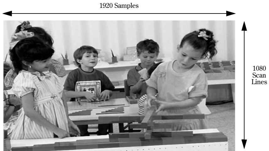
Figure 7.36. Scaling 4:3 Content for a 16:9 Display: “Wide” mode. Entire picture linearly scaled horizontally to fill 16:9 display, resulting in distorted picture unless used with anamorphic content.
