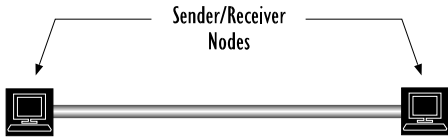
A point-to-point connection is direct.
