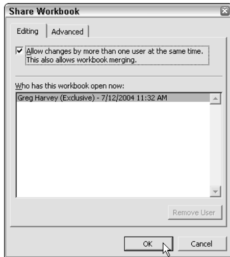
• Figure 41-1: Turning on file sharing by allowing changes by more than one user.
