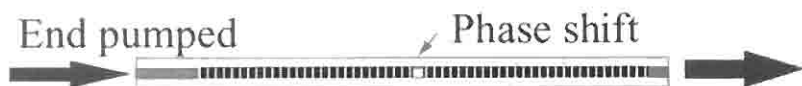
Figure 8.19: The EDFGL distributed feedback laser (EDFGL-DFB). The phase shift of \pi/2 forms a band pass in transmission.
