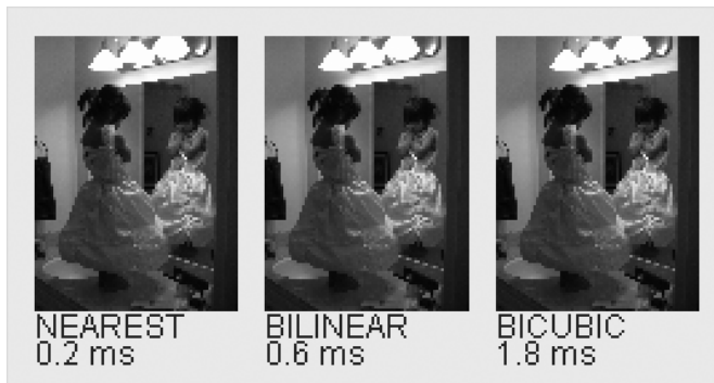
Figure 4-10 Close-up of the NEAREST , BILINEAR , and BICUBIC scaling results. All have similar artifacts for this large downscale.
