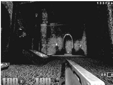
Figure 17-21 The bright-pass filter keeps only the brightest pixels.
