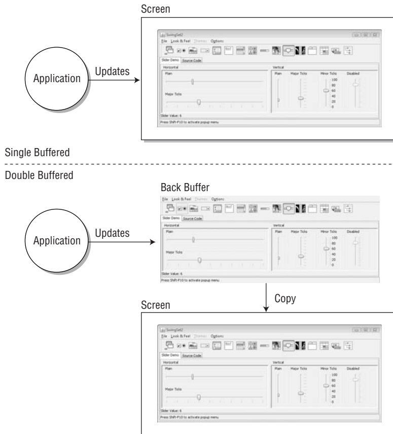
Figure 2-7 Single-buffered compared to double-buffered application.
