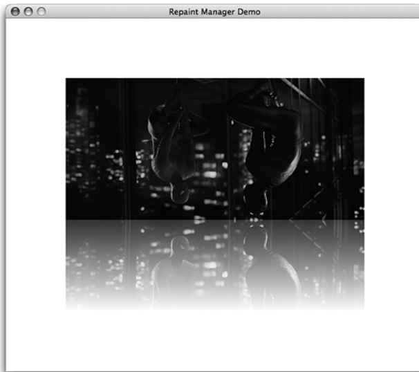
Figure 11-4 ReflectionPanel paints a real-time reflection effect for any child it contains.
