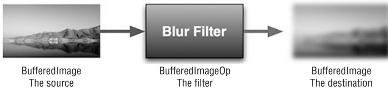
Figure 8-2 Filtering an image with Java 2D.
