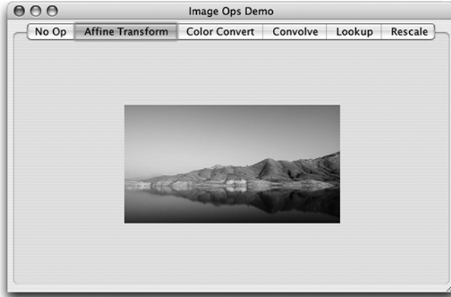
Figure 8-4 The size of the original image is reduced by 50 percent with an AffineTransformOp .
