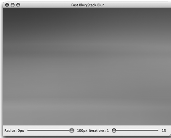
Figure 16-5 FastBlur with a radius of 100. The execution speed of this approach is independent of the radius size. But note that a blur with such a large radius makes the image impossible to recognize.
