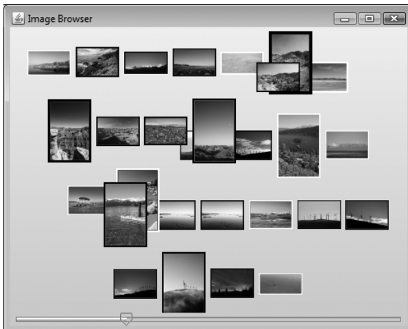
Figure I-7 Chapter 18, “Animated Transitions,” discusses automating animations between different states of a GUI. Here, a change in thumbnail sizes causes the pictures to automatically and smoothly animate to their new locations and sizes in the window.
