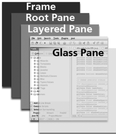
Figure 9-1 The glass pane sits on top of every other component in a Swing UI.
