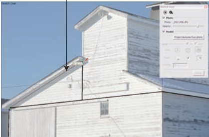
Color Plate 18: Using the endpoints of perpendicular edges to draw a diagonal (Chapter 7).
