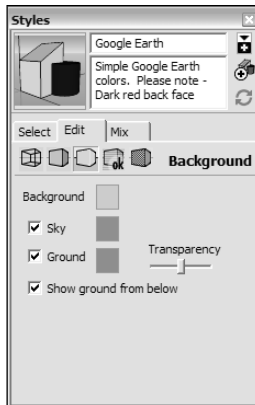
Figure 8-12: Use the Background tab to turn on the sky and the ground, and to choose colors.
