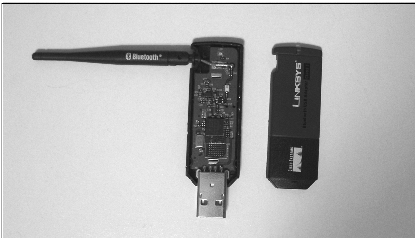
Figure 2.10 Opening the Bluetooth Adapter Case
