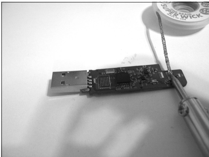
Figure 2.12 Preparing for the New Antenna
