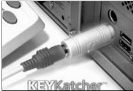
Figure 9.1 KeyKatcher with PS/2 Connectors
