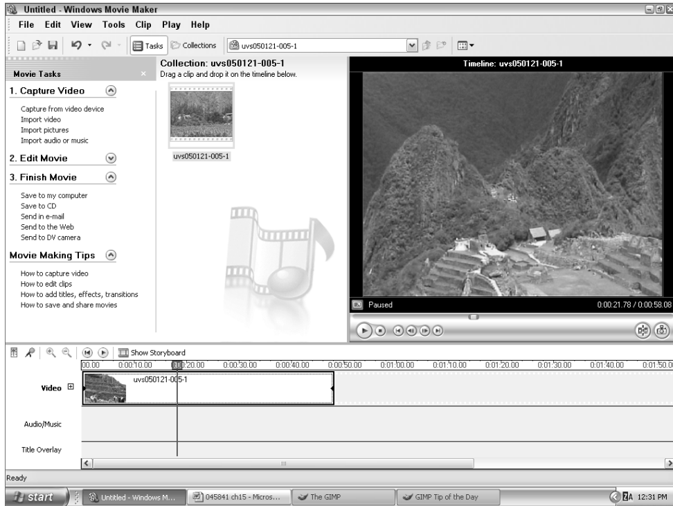
FIGURE 15-2: This screenshot shows the layout of the Windows Movie Maker screen. Note the timelines at the bottom of the screen.
