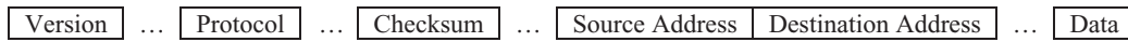
Figure 1: The header fields defined within an IPv4 datagram that are the most important to security and privacy.
