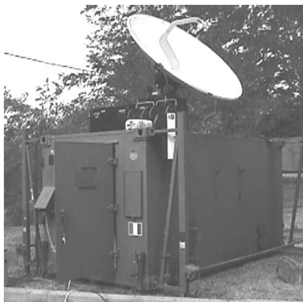
Figure 5: Milsat transportable station operating with commercial satellite. (Courtesy of Telespazio, Italy.)
