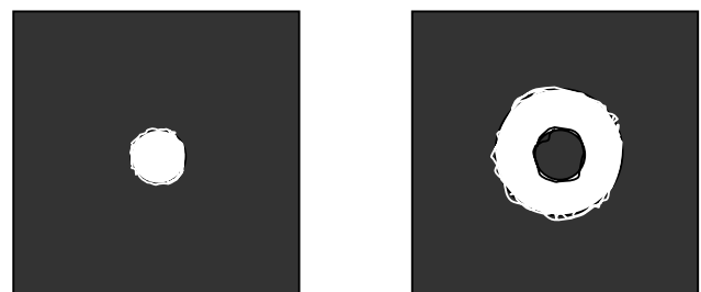
Figure 10: The 2D Mexican hat mother wavelet function in spatial domain (left) and in transform domain (right).
