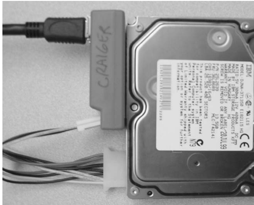
Figure 2: Write block with firewire connection.
