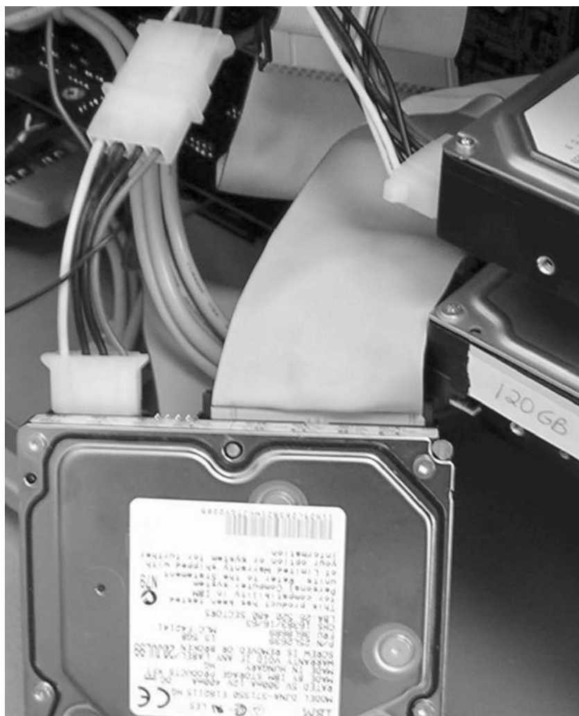
Figure 1: Direct connection to internal IDE controller.
