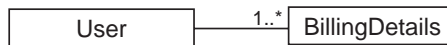
Figure 1.1 A simple UML class diagram of the user and billing details entities
