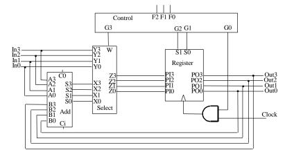
purpose register as designed in part 1 above. The "add to register" function is implemented in this design with a conventional four bit full adder as described in the lectures. The parallel input to the register is chosen by a multiplexer marked 'Select' The input to the register is either from the adder, if the select input W is 0, or from the external input (In0 .. In3) if the select input W is 1.
