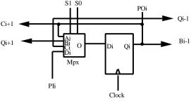
For a new application the Hold function is not required, but instead we need a clear function.
