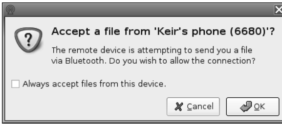
Figure 8-17. If you send files from a Bluetooth device to your PC, you may be asked to authorize receipt.
