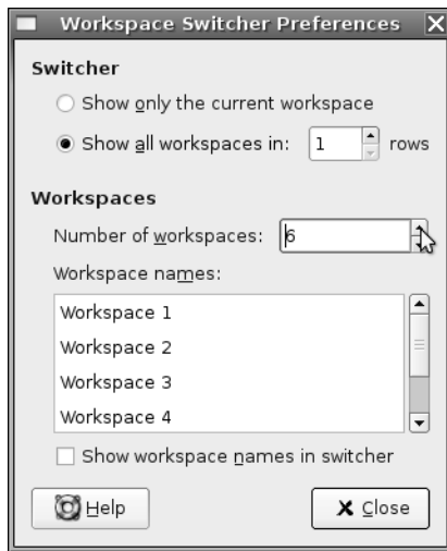
Figure 7-6. Four virtual desktops are set up by default, but you can have as many as 36.
