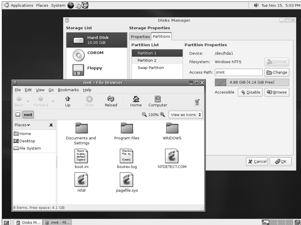
Figure 12-7. You can mount any partition, including those belonging to Windows, using the Disks Manager tool.
