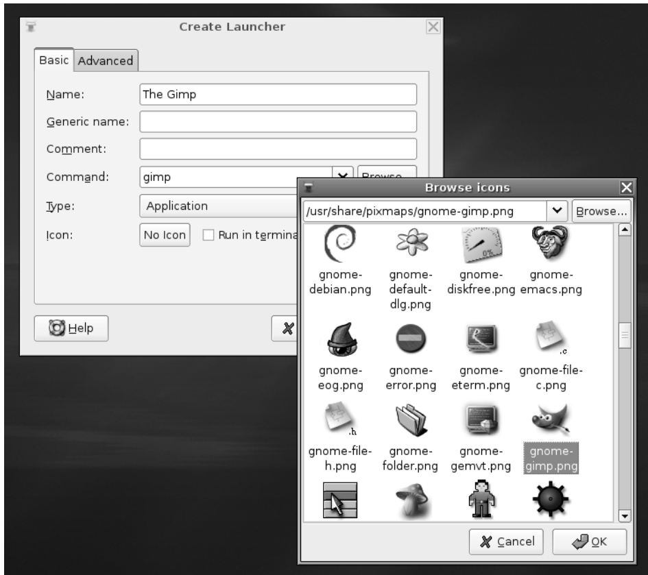
Figure 10-8. Creating a launcher is easy. Just fill in the Name and Command fields, and choose an icon.
