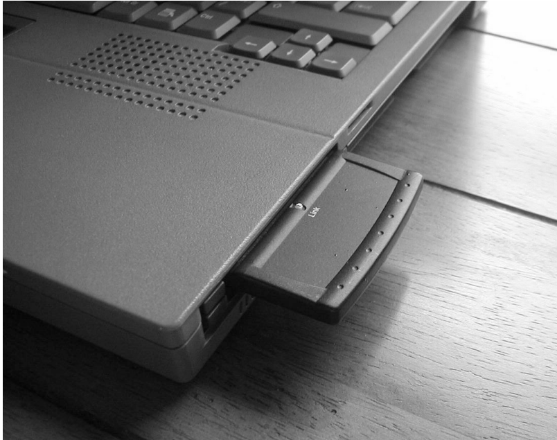
Figure 8-3. If you use a PCMCIA wireless card, it will most likely have an external antenna.
