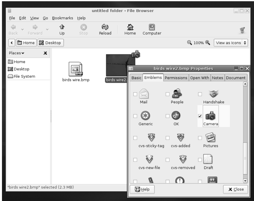
Figure 12-5. A variety of miniature emblems can be applied to an icon to aid recognition of the file.
