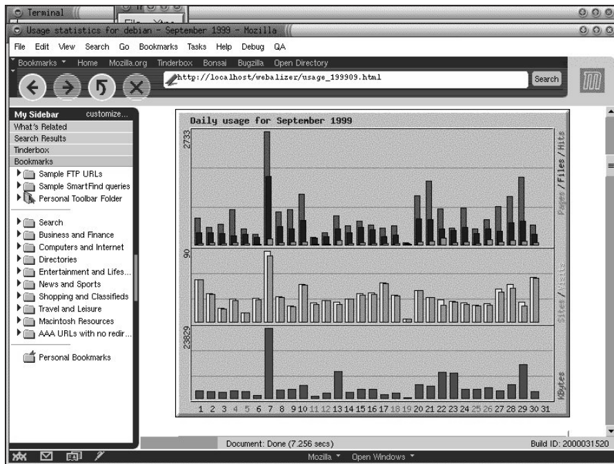
Figure 21-2: Webalizer creates graphical charts from the log file data, such as this one that shows usage for one month.
