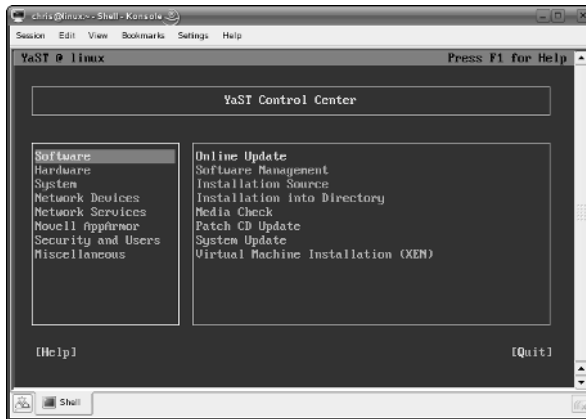
Figure 10-2: Use the arrow and Tab keys to navigate YaST in text mode.
